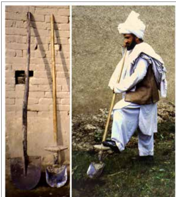
Figure 12. Digging implements, Village Bharat. Left: a shovel ( belcha ) and foot shovel ( yūm ); right: demonstrating the use of a yūm . Photographs by the author.
