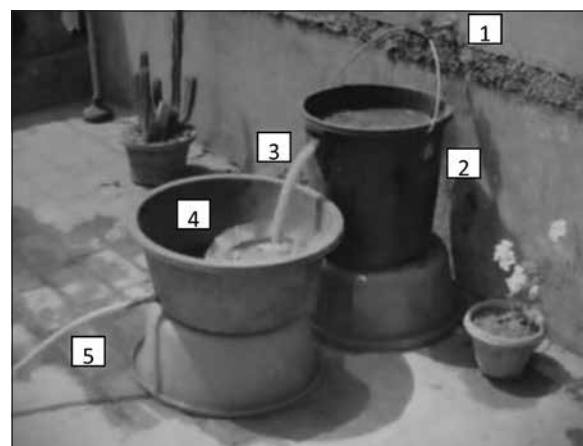
Figure 5. Flotation equipment for the recovery of charred plant remains from samples of deposits from the site of Sheri Khan Tarakai. Key: 1: Fresh clean water supply; 2: Flotation 'tank'; 3: Overflow pipe carrying floated material away from the 'tank'; 4: Nest of sieves (mesh sizes 1.0 and 0.5 mm) collecting the floated material; 5: Pipe carrying away used water and fine sediments to drainage system.
