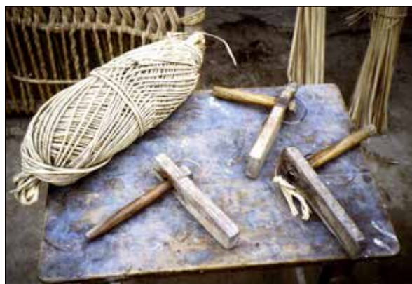
Figure 6. A coil of rope made from leaves of Munja and the hand-held gadgets ('karkare') which are used to twist the leaves into rope, as described in the text. Bharat Village.
