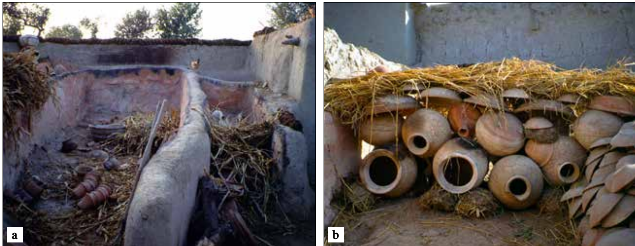
Figure 9. Workshop kilns. (a) A double kiln in the courtyard of Gul Nawaz (village Nurar), the larger one (7.8 m long x 3.0 m wide and from 0.4 m to 0.8 m high) is for firing a range of pots, while the smaller one (3.8 long x 2.0 m wide and from 0 m to 0.45 m high) is used for firing thaibi . (b) When stacking his dried pots for firing, Umar Khan (village Mandeo) places a layer of dung cakes on the bottom of the kiln with the pots carefully stacked on top, with bits of dung cake packed into the spaces between them. Flat dishes are placed on the top and over these a final layer of straw (note: this was reconstructed as a demonstration, using already fired pots).
