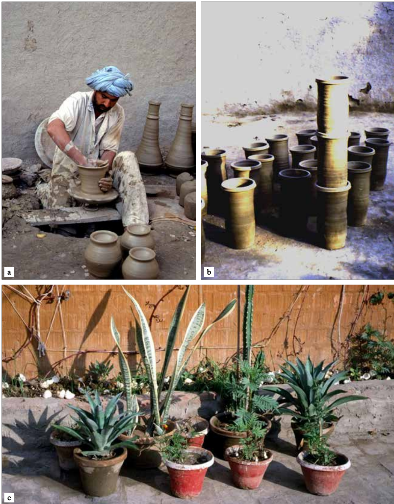
Figure 13. Other popular ceramic items. (a) Habibullah Khan (village Nurar) at his foot/kick wheel throwing the body of a hubble-bubble pipe ( chillum ), finished examples of which are drying behind him. (b) Pottery drainage pipes made by Habibullah Khan. (c) Terracotta flower pots; see also Figure 6(c).
