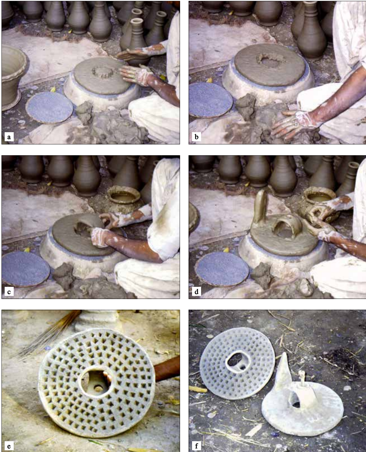
Figure 6. Sequence showing Habibullah Khan (village Nurar) making a rice-husking mill, or dhalinā . (a) Preparing the main body into which (b) is made a central hole. (c) A band of clay forms an arch over the central hole, (d) a small hole in made in the top of this arch (to hold the wooden peg around which the finished mill will rotate) and a handle is attached to the outer edge of the main body. (e) When partly dry, numerous diamond-shaped holes incised in a regular pattern into the base of the body produce the milling surface. (f) After firing, the dhalinā is ready for use as a rotary husking mill.
