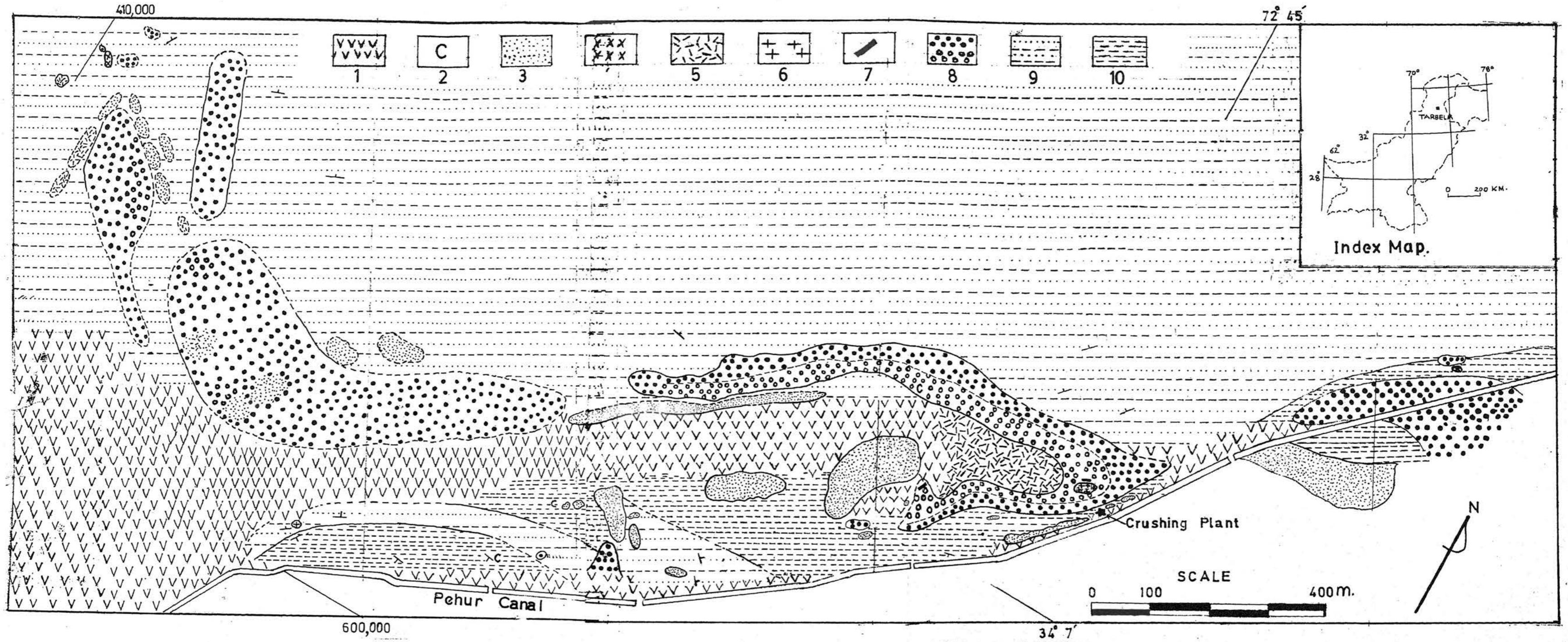
Fig. 1. Geological map of the Tarbela alkaline complex (1) Overbarden/alluvium, (2) Carbonatite intrusions, (3) Albitecarbonate breccia, (4) Granites, (5) Albitites (including carbonate, quartz and pure albitites), (6) Amphibole Albitites, (7) Dolerite dykes, (8) Gabbroic intrusions: a-Melanocratic, b-Leucocratic, (9) Tanawal Formation, (10) Salkhala Formation.
