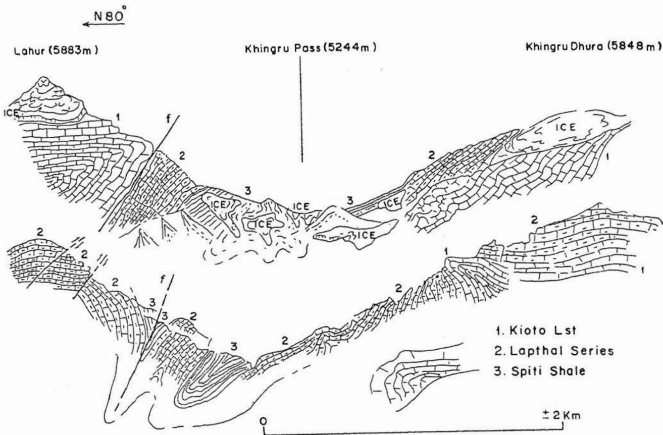
Fig. 7. Inverted fold structures in the complicated limbs of Chidamu-Lapthal Syncline.
