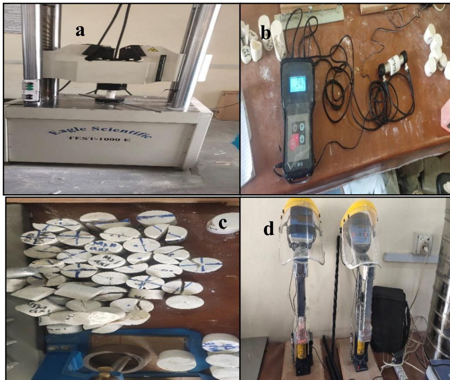
Fig. 4. Experimental setup (a) Universal testing machine (b) Ultrasonic pulse velocity tester (c) Marble sample (d) Point load index
