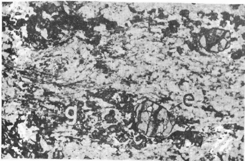
Fig. 3. Photomicrograph showing garnets of two generations in Manglaur crystalline schist; fresh euhedral crystals (e) growing across earlier crushed granoblasts (g). (Field 2.3 x 3.3 mm).
