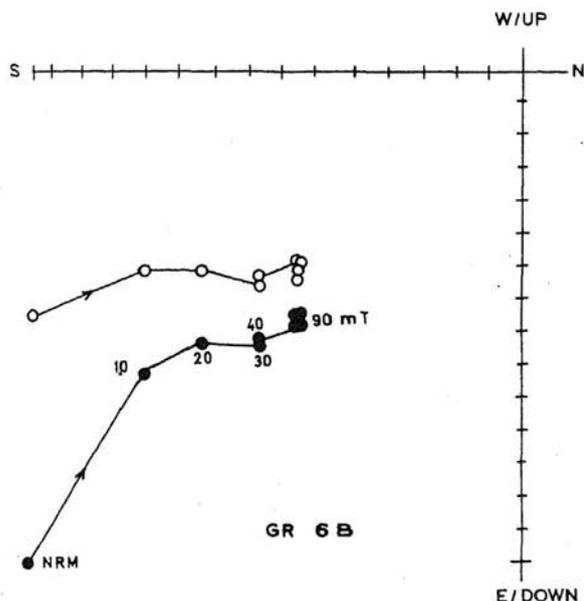
Fig. 1. Orthogonal projection diagram of AF demagnetization. Open (solid) circles represent projection of end points of demagnetization vectors on vertical (horizontal) planes. Intensity units are  $10.4 \text{ A/m}$ .
