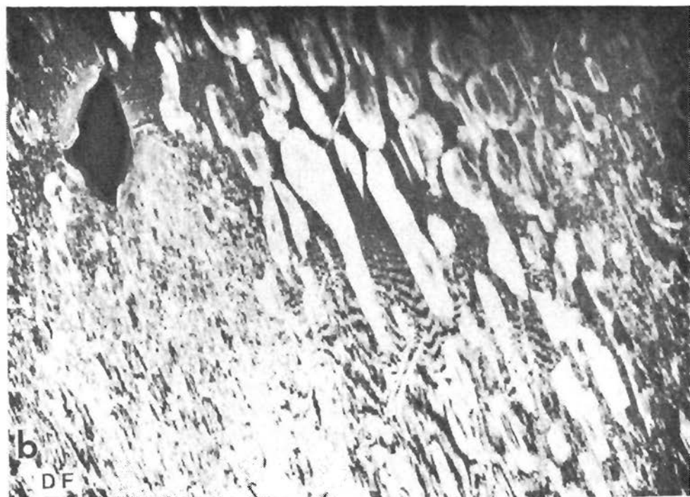
Fig. 2. (a) BF and (b) DF images of lath-like defects in calcite grain in siderite from Erzberg.
