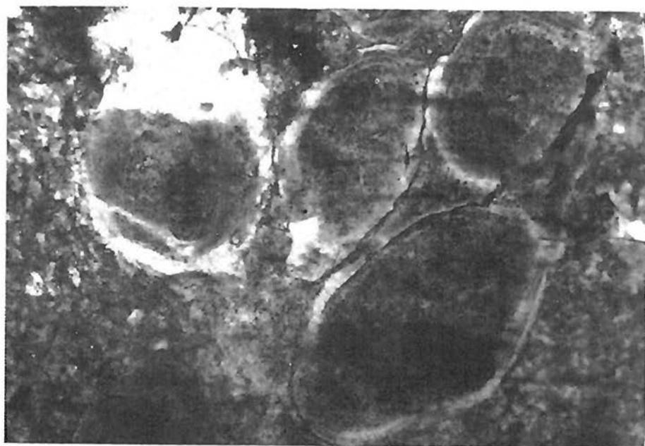
Fig. 3. Photomicrography showing uniform distribution of oval shaped pellets (Plane Light, x 25).
