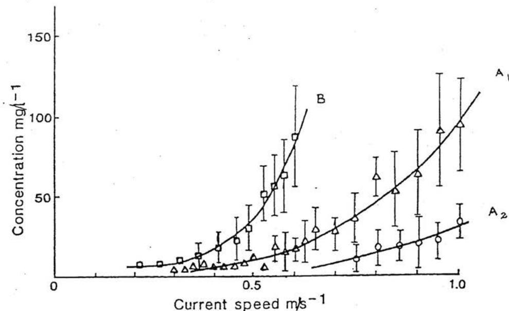
Fig. 5. Relationship between current velocity and suspended load concentration. Concentrations are nearly equal at A and B despite difference in current velocity, suggesting the presence of mud at A.  $A_1$  and  $A_2$  are pre- and post-storm concentrations at site A. Bars are 1 standard deviation.
