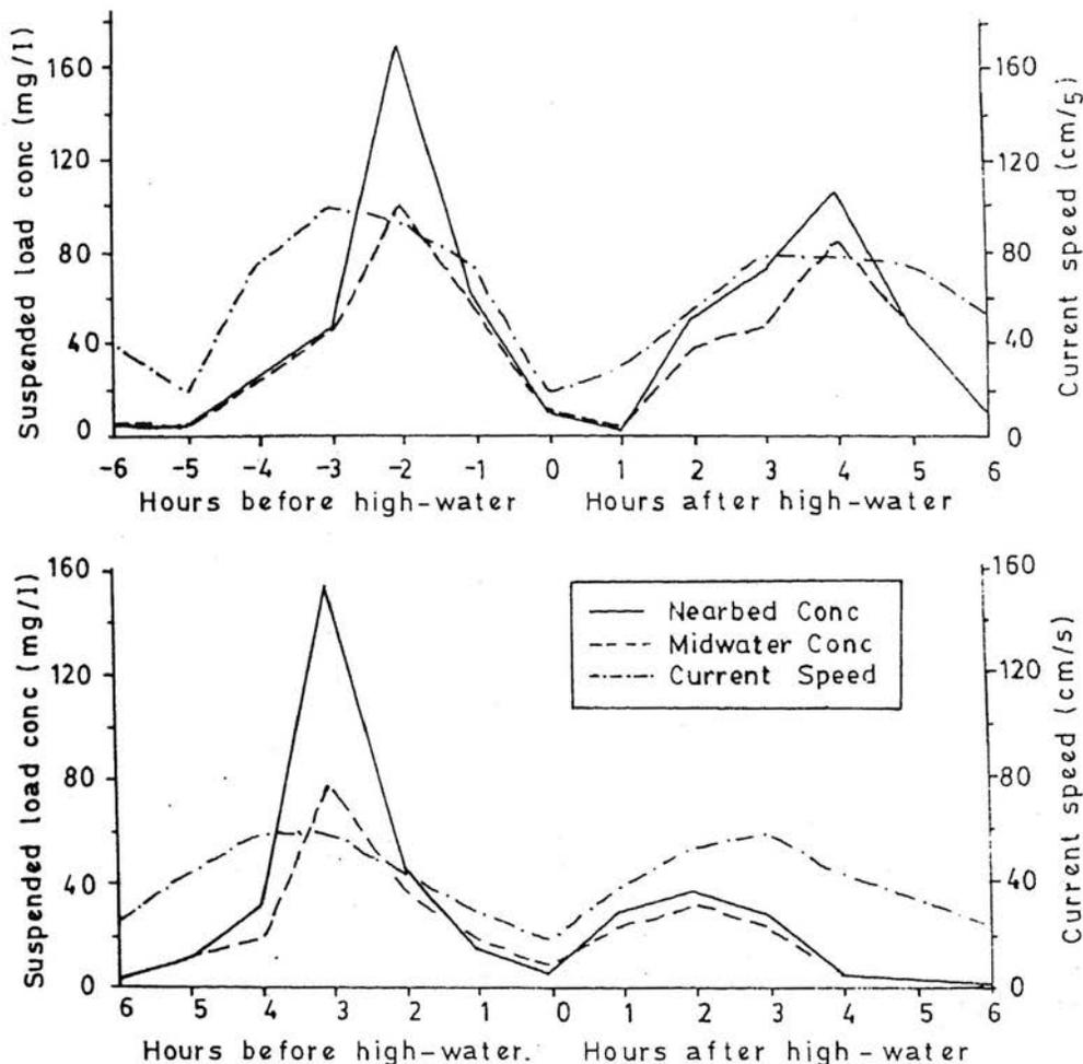
Fig. 7. Variation in the suspended load flux during a 13 hour semi-diurnal tidal cycle for spring tides; (a) station A, (b) station B. At both stations the fastest currents are experienced around 3 hours before the high water.
