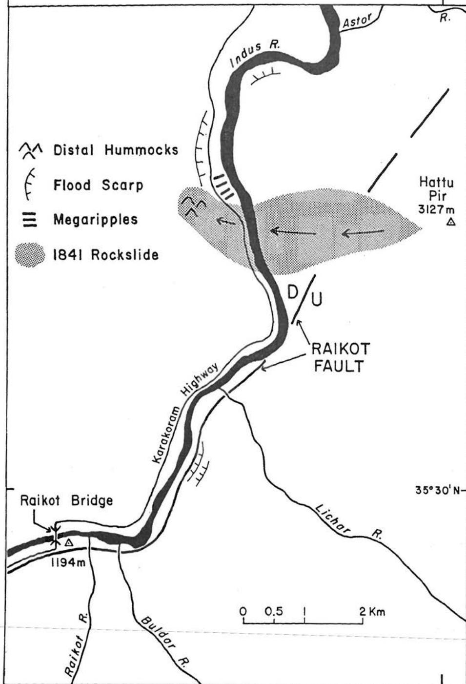
Fig. 6. Sketch map of the rockslide that blocked the Indus River in 1841. The massive slope failure from Hattu Pir was produced by an earthquake, presumably from movement on the Raikot fault that crosses beneath the slide.
