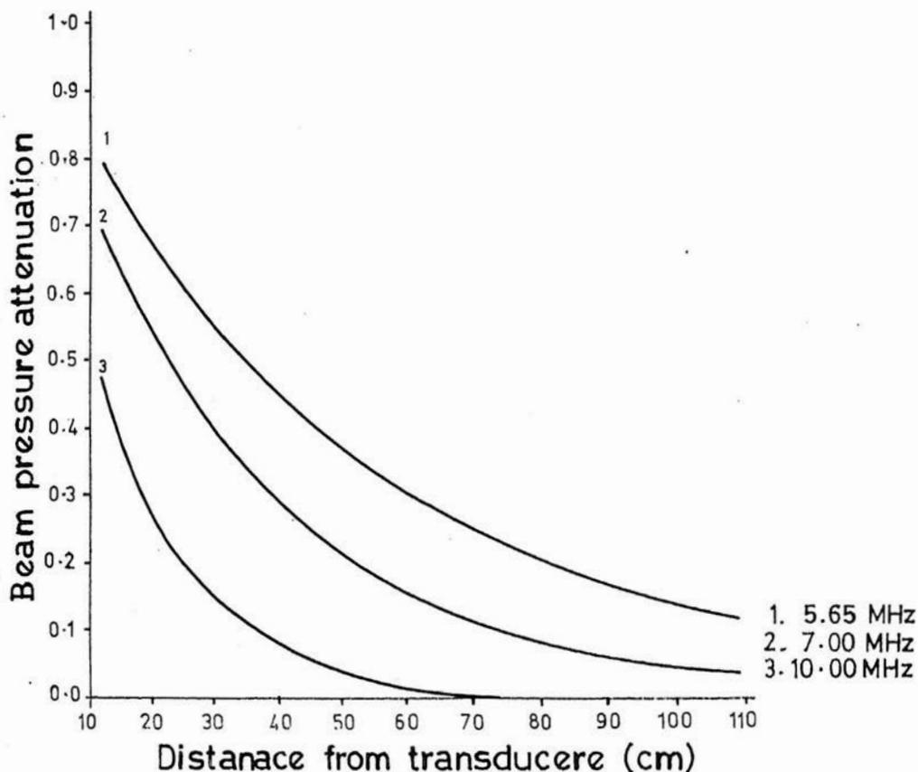
Fig. 1. The effect of beam pressure attenuation (due to water) in a two-way transmission on different frequencies.
