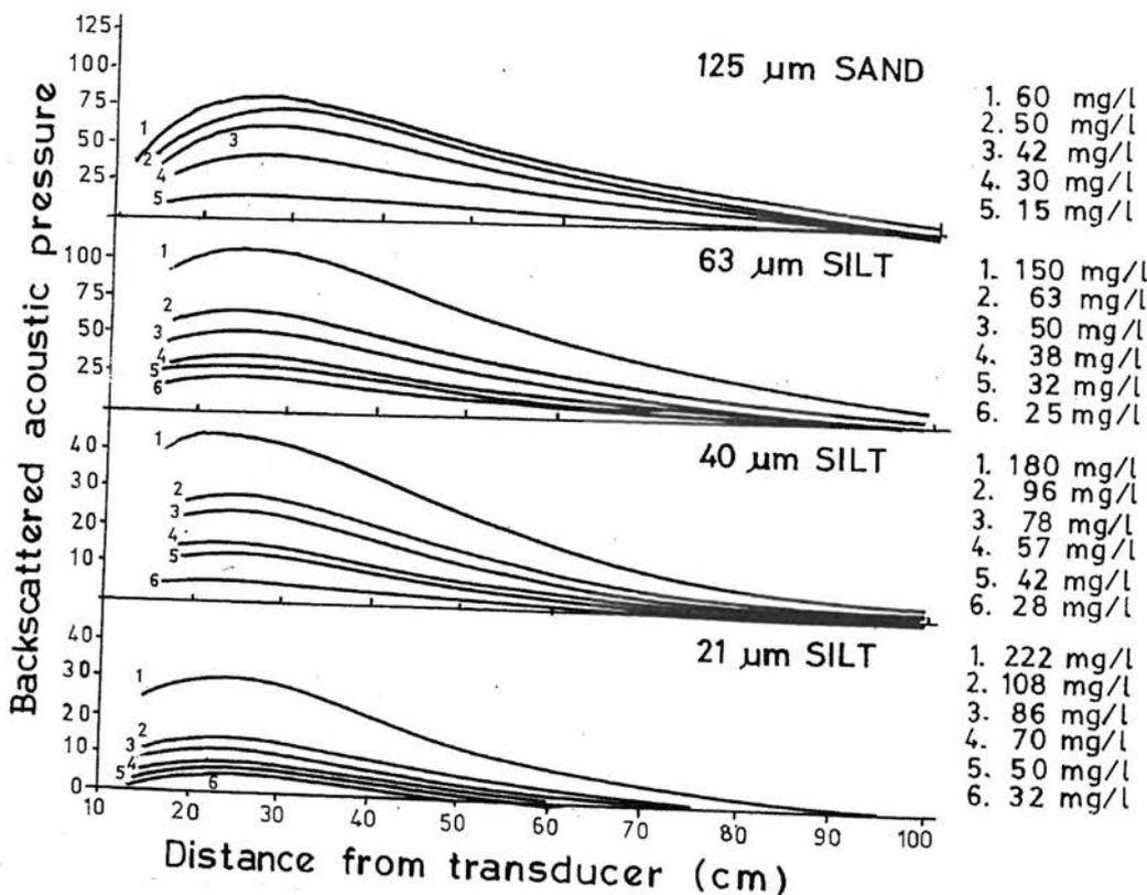
Fig. 4. Profiles of suspended sediment in the tank during calibration exercises. (a) values of backscattered pressure ( $P_b$ ) from 5.65 MHz frequency.
