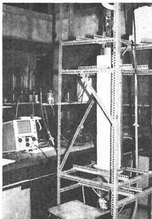
Fig. 3. Photograph showing the cylindrical tank, the pump, the external hose and ABM for laboratory calibration.
