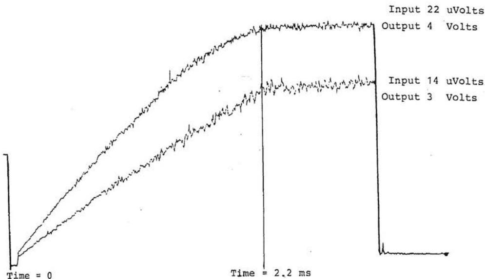
Fig. 2. Time Variable Gain (TVG). The amplitude of backscattered signal increases with time from 14 and 22 micro-volts to 3 and 4 Volts, respectively in a matter of 2.2 millisecond.
