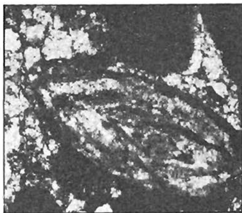
Fig. 10 (right). Photomicrograph (crossed nicols) of a nummulites shell surrounded by sparry calcite. Conglomerate from the Chaudhwan Formation.
