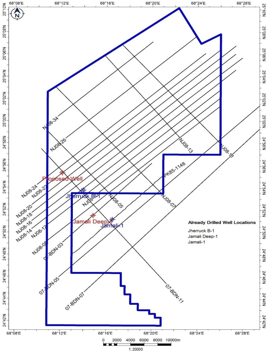
Fig. 1. Base map of study area displaying seismic dip and strike lines along with drilled well and proposed well location.
