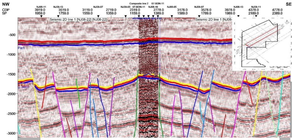
Fig. 8. Composite of Seismic lines NJ08-14, BDN-11 and NJ08-22.
