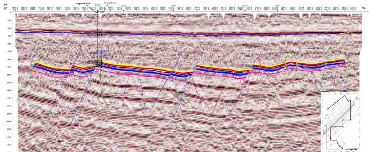
Fig. 6. Dip line NJ08-14 with interpretation, well tops of Jherruck-B1 well and proposed new well location.
