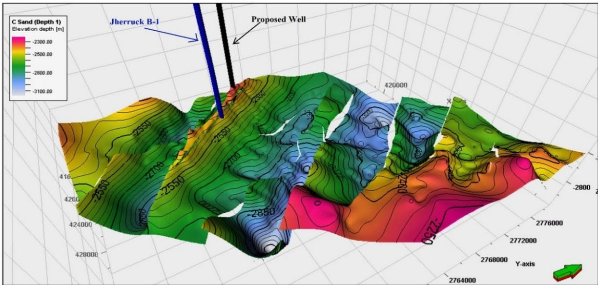
Fig. 14. Depth Contour map of C-Sand along with location of drilled well Jherruck-B1 and proposed well.
