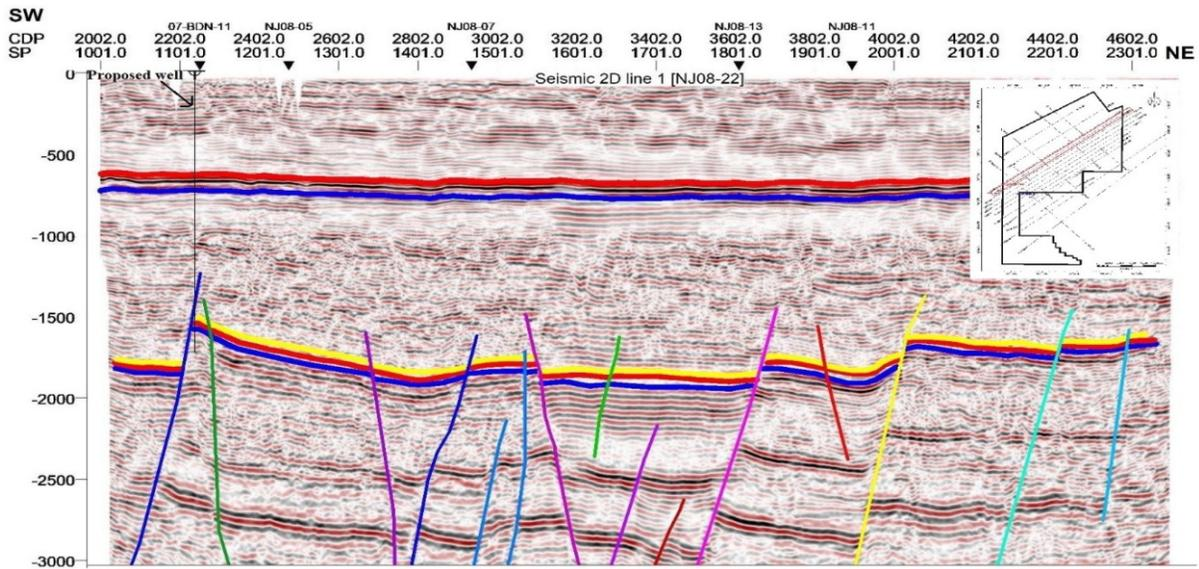
Fig. 10 Interpreted Seismic line NJ08-22 with proposed well location.
