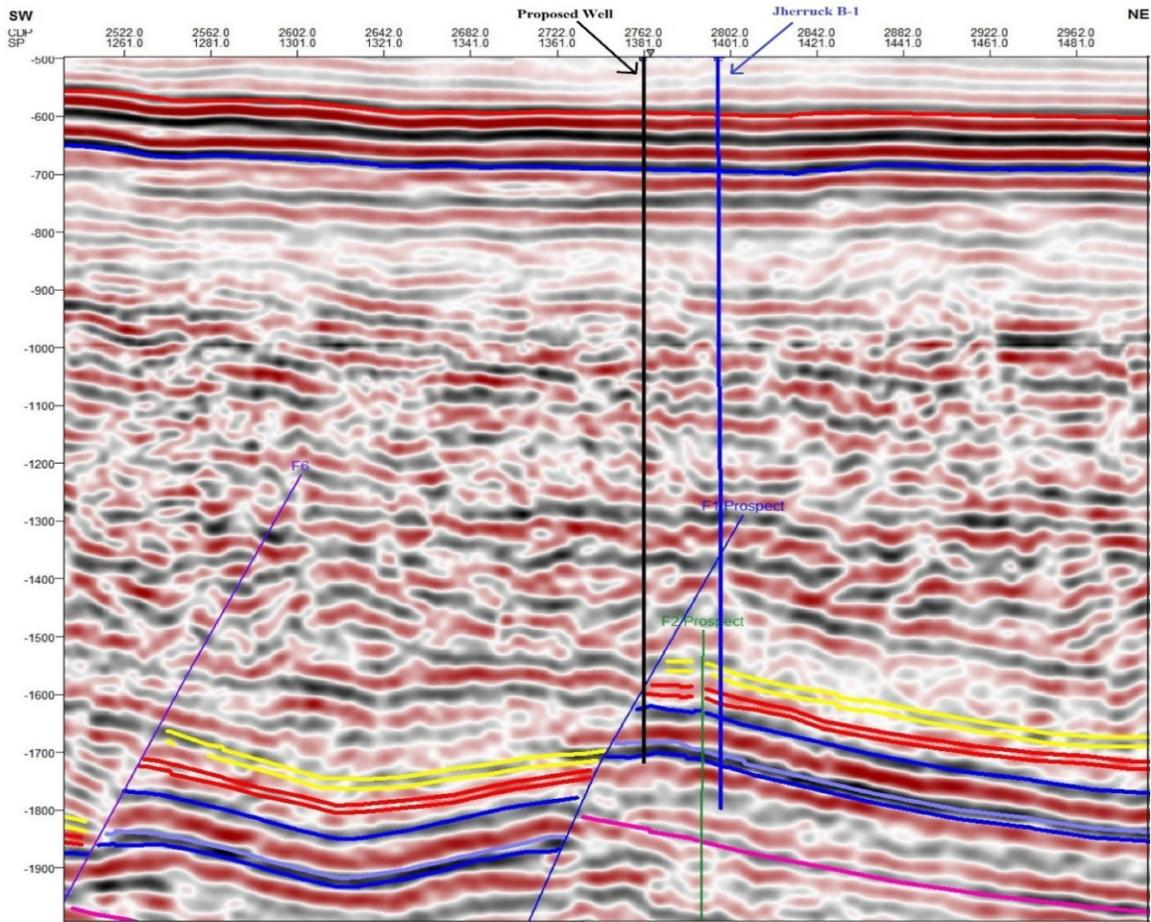
Fig. 7. Enhanced/zoomed image of Dip line NJ08-14 with interpretation and location of existing well Jherruck-B1 and proposed new well location (Projected on this line).
