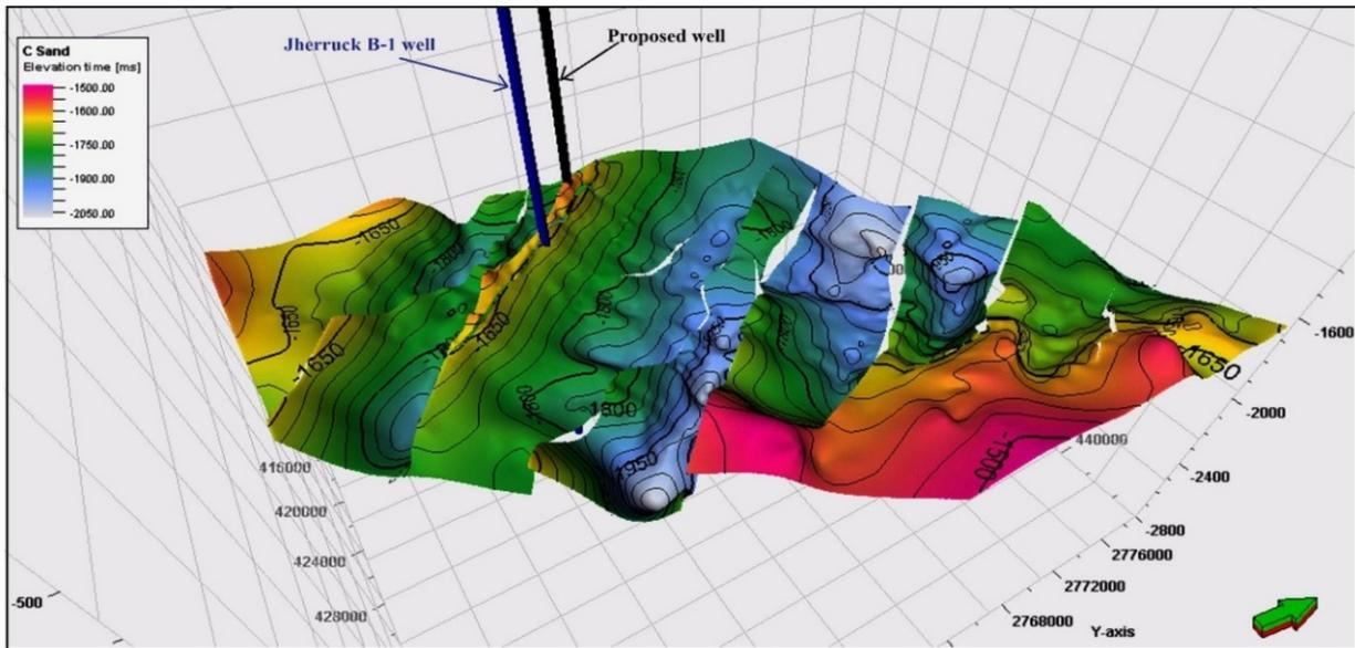
Fig. 13. Time contour map of C-Sand along with location of drilled well Jherruck-B1 and proposed well.
