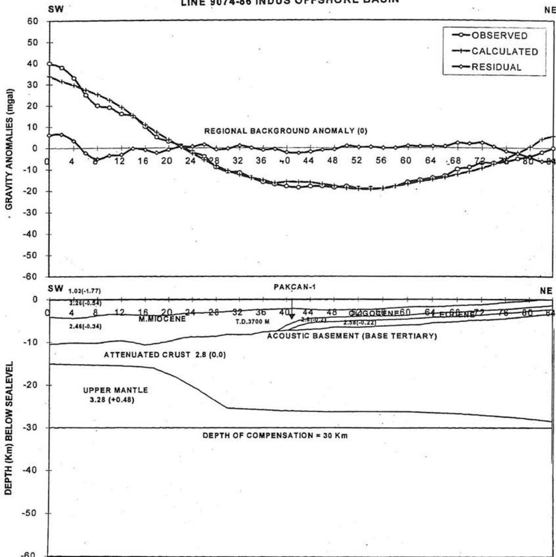
Fig. 7. Depth model and gravity anomalies(composite) along the line 9074-86 (Indus Offshore Basin) as determined from limited seismic reflection data and gravity observations, by assuming zero regional background anomaly.
