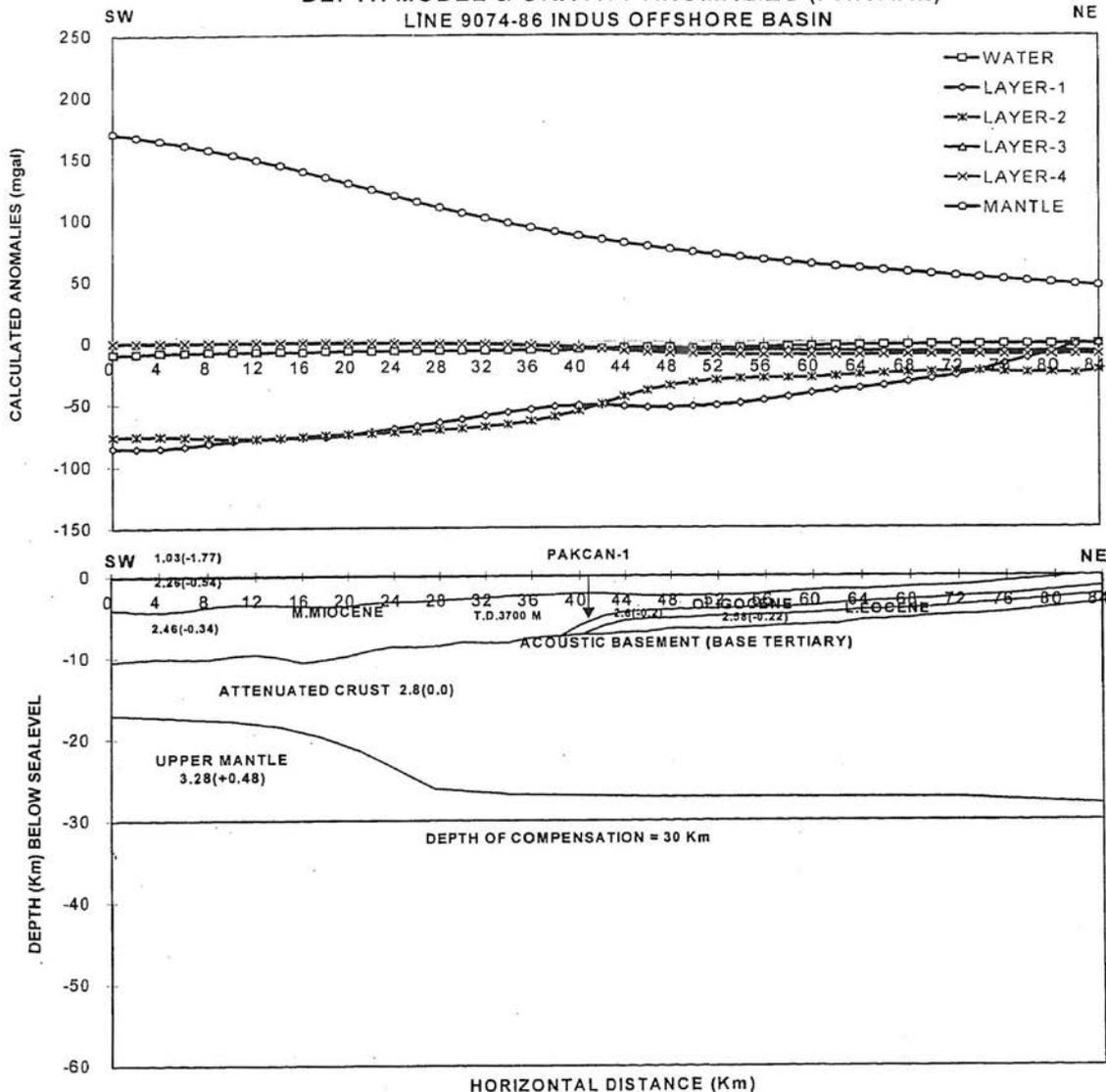
Fig. 10. Depth model and calculated gravity responses for individual layers along the line 9074-86 (Indus Offshore Basin) by assuming zero regional background anomaly.
