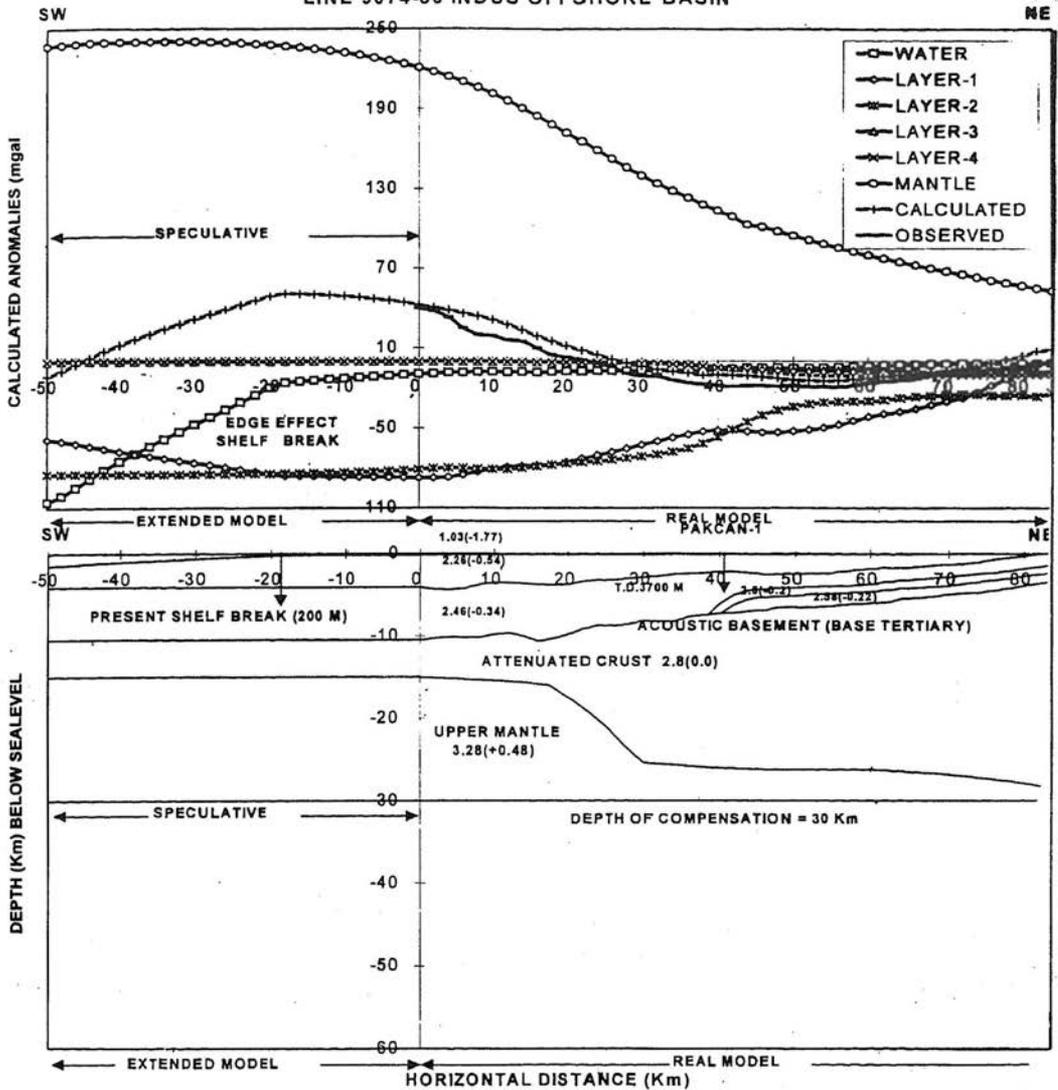
Fig. 14. Speculative true scale depth model (bottom) and calculated gravity responses for individual layers (top) along the line 9074-86 (Indus Offshore Basin). The model from 0 to -50 km mark is projected from the right half except for the seabed configuration which is plotted using true values.
