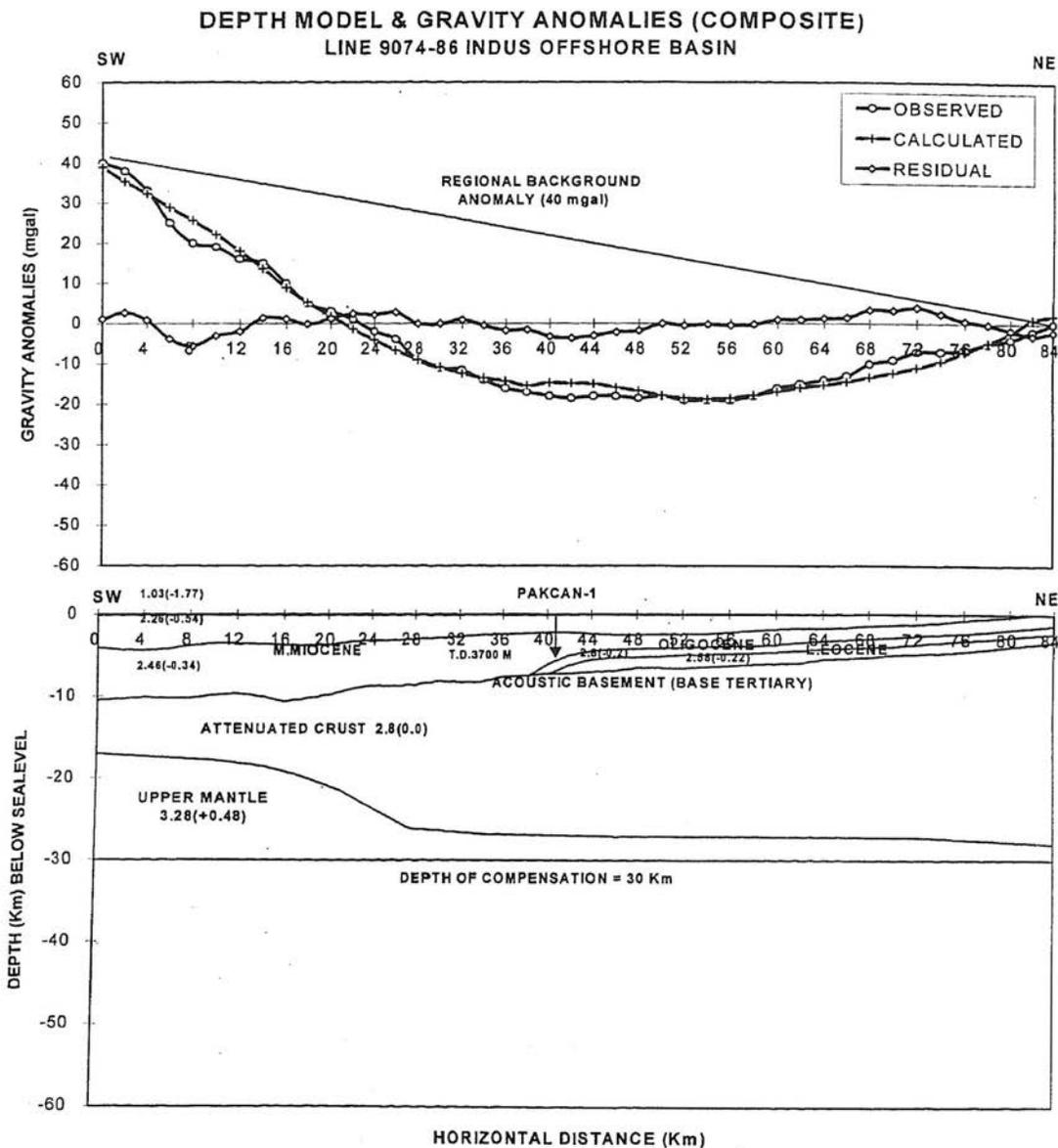
Fig. 9. Depth model and gravity anomalies (composite) along the line 9074-86 (Indus Offshore Basin) as determined from limited seismic reflection data and gravity observations, by assuming 60 mgal (60, -0.7143) regional background anomaly.
