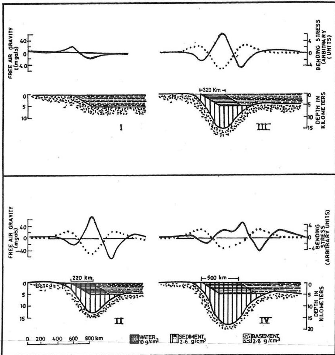
Fig. 3. Calculated gravity (free-air) anomalies and relative bending stresses (dotted) for flexural models of different load widths. Only the upper part of the models are shown, the base of the crust is included in the gravity calculations (After Walcott, 1972).
