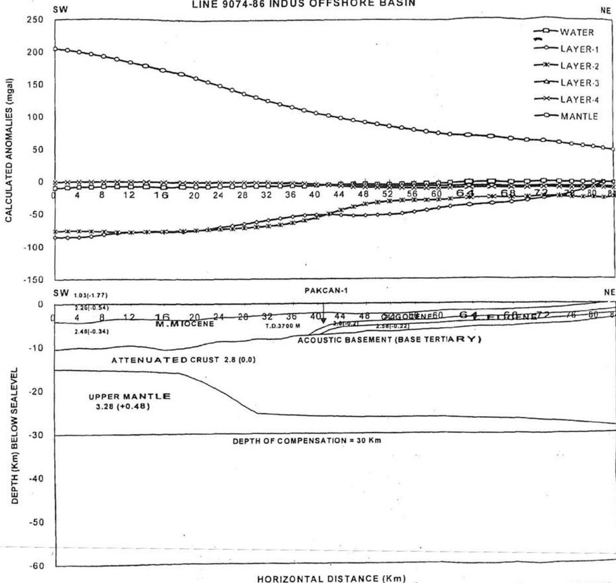
Fig. 11. Depth model and calculated gravity responses for individual layers along the line 9074-86 (Indus Offshore Basin) by assuming 40 mgal (40, -0.4762) regional background anomaly.
