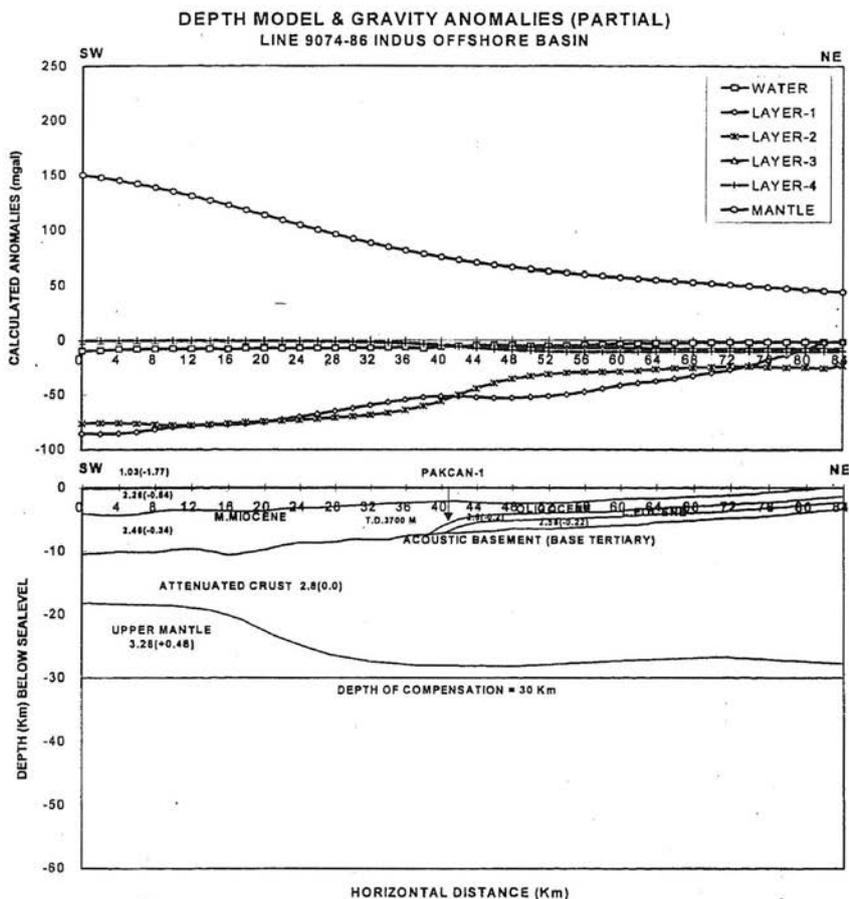
Fig. 12. Depth model and calculated gravity responses for individual layers along the line 9074-86 (Indus Offshore Basin) by assuming 60 mgal (60, -0.7143) regional background anomaly.
