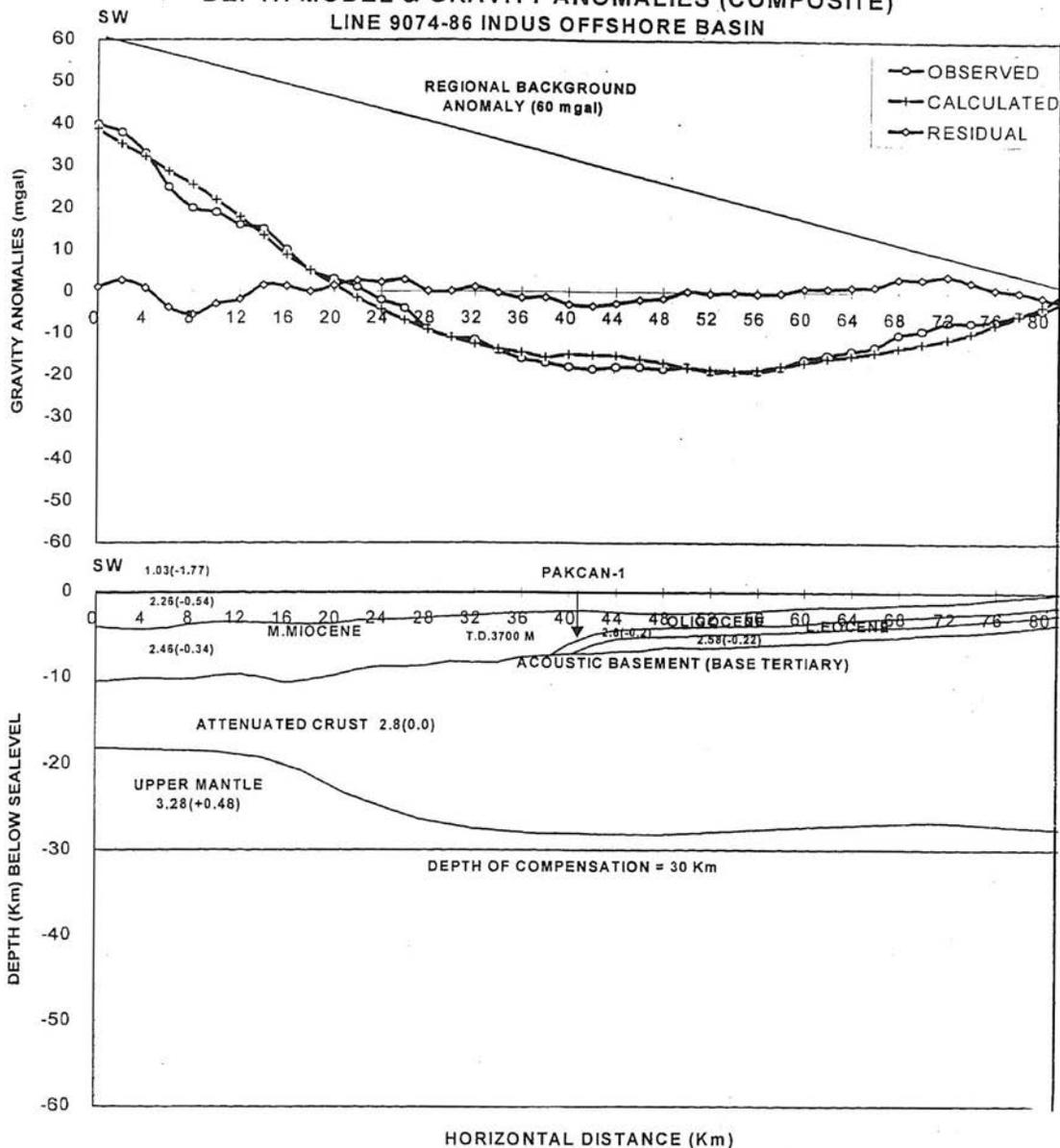
Fig. 8. Depth model and gravity anomalies (composite) along the line 9074-86 (Indus Offshore Basin) as determined from limited seismic reflection data and gravity observations, by assuming 40 mgal (40, -0.4762) regional background anomaly.
