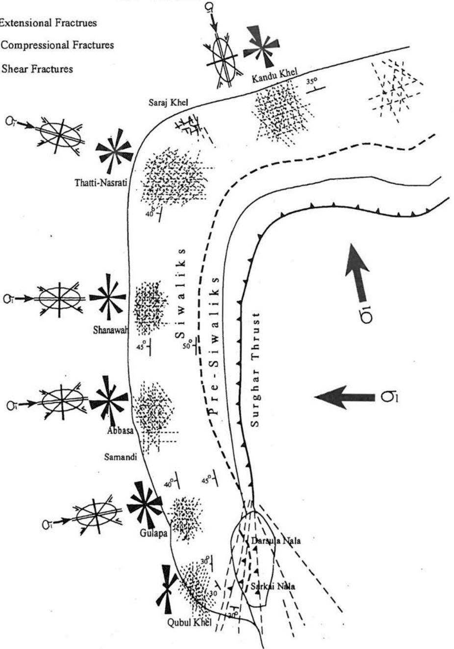
Fig. 9. A preliminary structural map of fractures recorded in the Siwalik Group at different stations, illustrated by rose and stress diagrams, Surghar-Shinghar Range, Bannu Basin.
