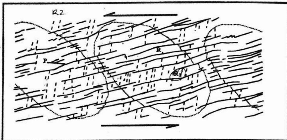
Fig. 5. Sinistral simple shear in a clay block model induced by shearing the substrate of the clay. Note the formation of  $R_1$  and  $R_2$  Riedel fractures (after Twiss & Moores, 1992).
