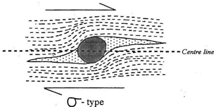
Fig. 6a.  $\sigma$ -type porphyroblast, showing sense of shearing. Note the tails do not cross the line parallel to the foliation through the centre of the grain (Twiss & Moores, 1992).
