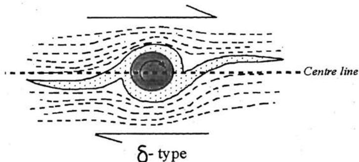
Fig. 6b.  $\delta$ -type porphyroblast, derived from the rotation of  $\sigma$ -type. Note the tails do cross the central line (Twiss & Moores, 1992).
