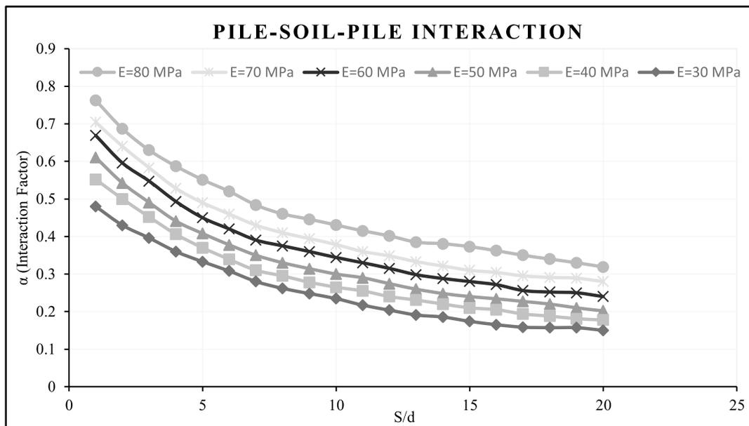
Fig. 6. Comparison of Interaction factor for varying  $E$ , and  $s/d$
