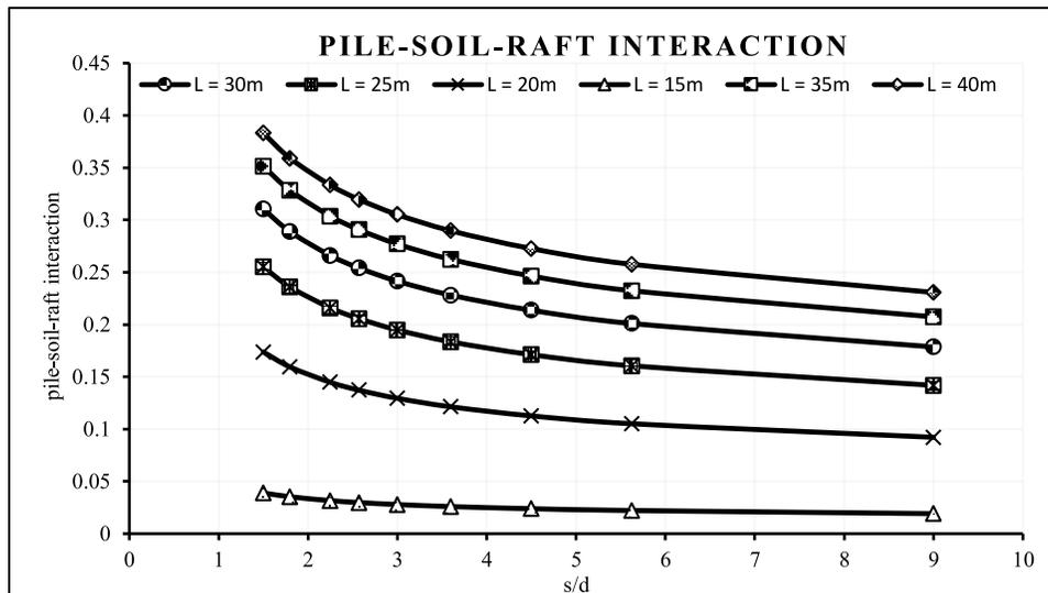
Fig. 11 Interaction factor  $r_p$  with  $s/d$  for different length
