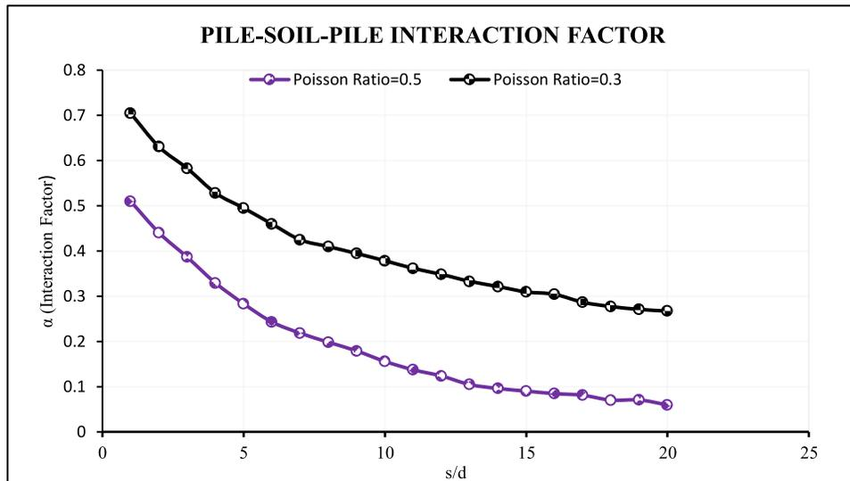
Fig. 8 Variation of s/d for Poisson's ratio of 0.3 and 0.5 at E= 70 MPa
