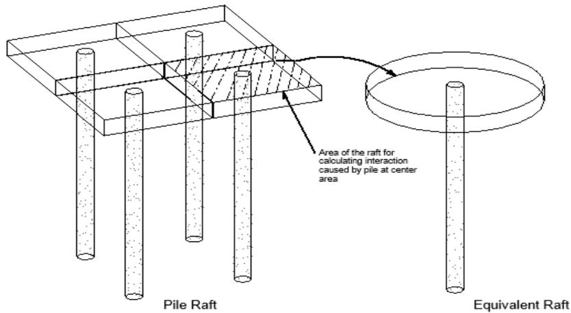
Fig. 10 Equivalent raft Concept.
