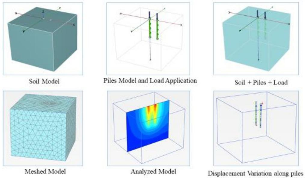
Fig. 1 Model construction for analysis in Plaxis 3D
