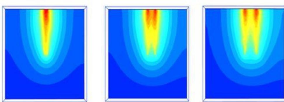
Fig. 5 (a) shows overlap of pressure bulb when piles are at distance of 2m (b) shows overlap of pressure bulb when spacing is 6m (c) shows overlap of pressure bulb when spacing is 9m between piles
