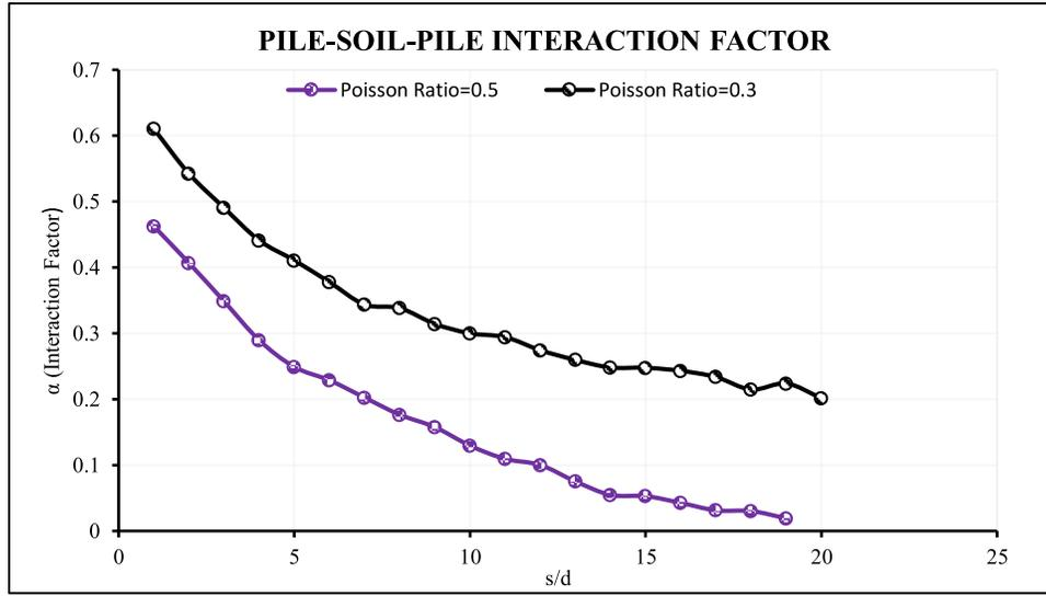
Fig. 9 Variation of s/d for Poisson's ratio of 0.3 and 0.5 at E= 50 MPa
