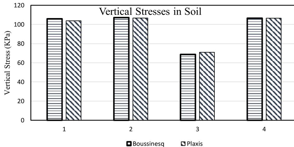
Fig. 3 Comparison of vertical stress obtained through PLAXIS 3D and Boussinesq Equation
