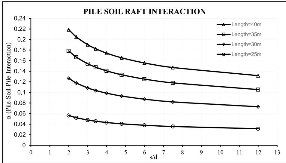
Fig. 12 Variation of Interaction factor with  $s/d$  for different length
