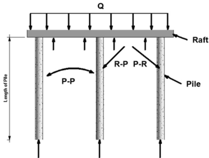
Fig. No. 1 Pile-Soil-Pile and Pile-Soil-Raft Interaction
