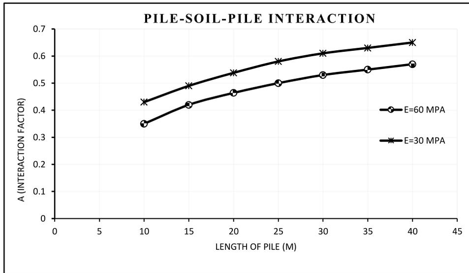
Fig. 7 Comparison of Interaction factor for varying length and E
