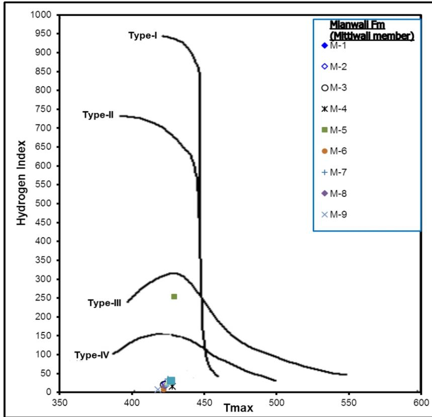
Fig. 4. HI versus Tmax showing kerogen types in the studied samples.
