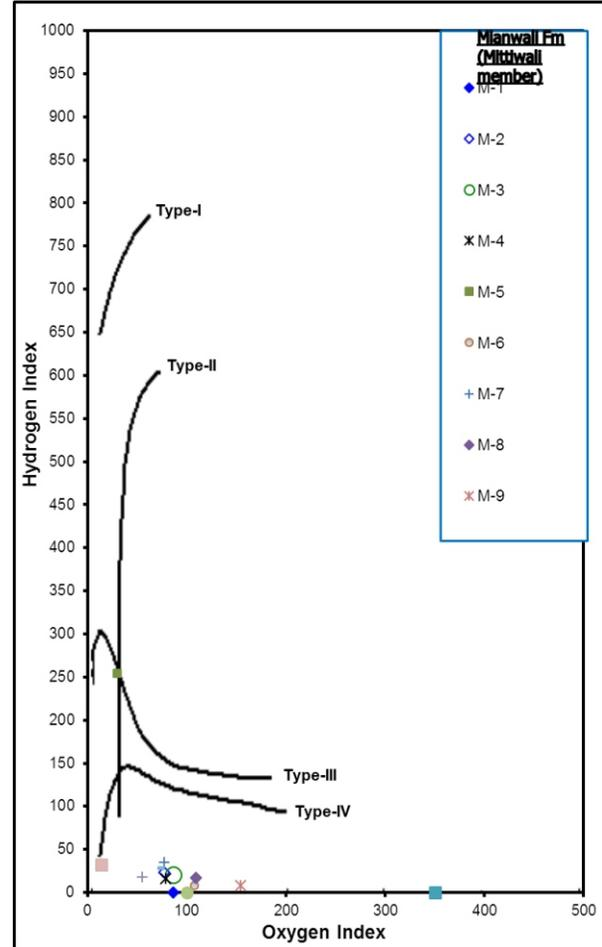
Fig. 2 Van Krevelen's diagram showing types of kerogen in the studied samples.
