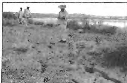
Photo 12. Margin of a stable sand dune with fractures in response to lateral spreading liquefaction.
