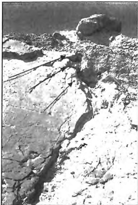
Photo 5. The Cracks/Joints of the Litra Formation do not Penetrate the Boulder Cover
