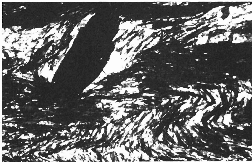
Fig. 11. Relict S_1 as intrafolial folds in dominant S_2 foliation. Rotation of magnetite grain can also be seen. Graphitic phyllite containing also quartz, muscovite and graphitic dust. Crossed polars, field of view 1.8 mm long.
