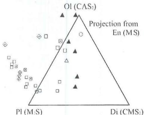
Fig. 9. Compositional variation of rocks from the SQUC shown in a projection from MS into  $M_2S-CAS_2-CMS_2$  plane of the CMAS quadrilateral of Cawthorn & O' Hara (1976). Ol=Olivine; Pi=Plagioclase; Di=Diooside
