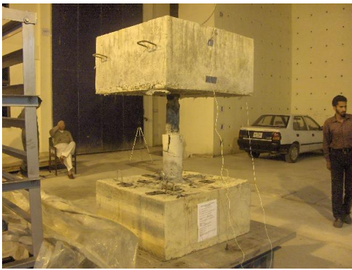
Fig. 9. 1 st shake table test of RC bridge pier conducted in November 2006.
