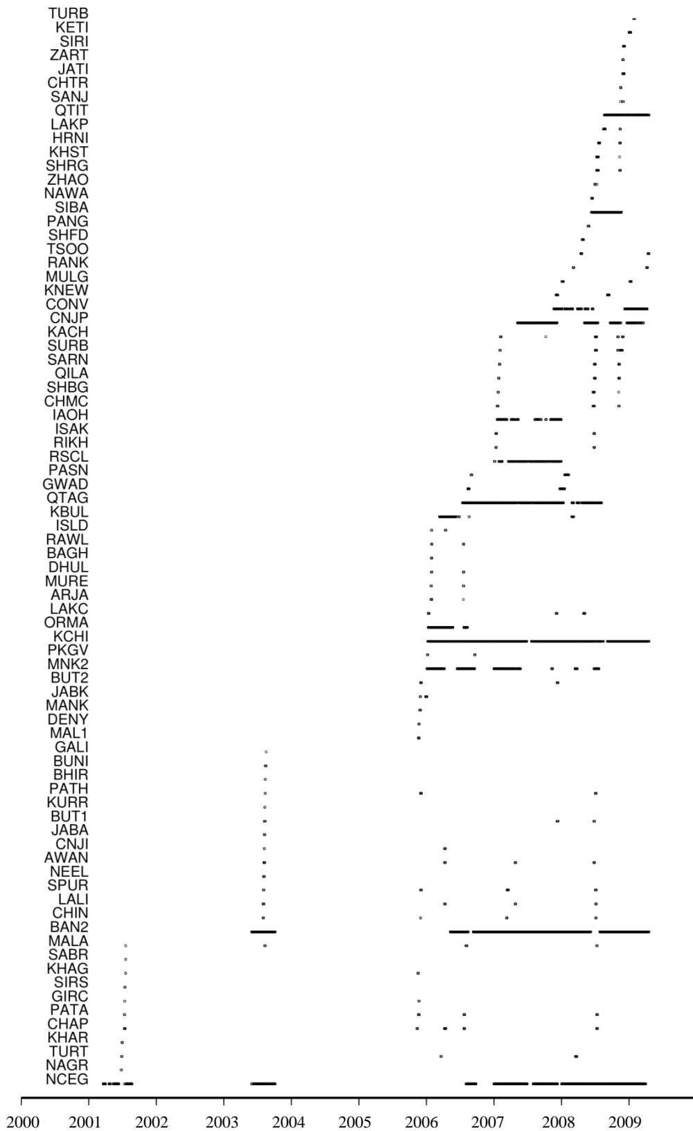
Fig. 1. The summary of TriGGnet in Pakistan showing GPS points (y-axis) and their measurement history (x-axis) between 2001 and 2009. Points with solid horizontal black line are the permanent stations while those with dots are reoccupied after every 2 to 3 years with measurements for a minimum of three days.
