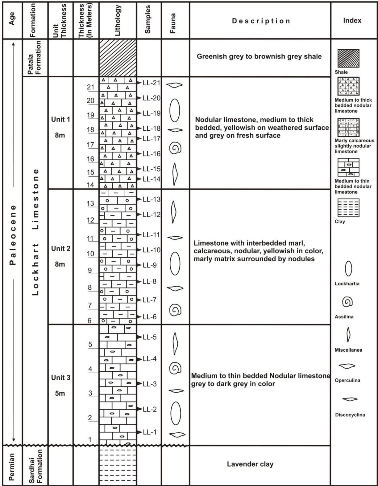
Fig. 2. Lithological log of the measured section of Lockhart Limestone in the Nilawahon Gorge, Central Salt Range.
