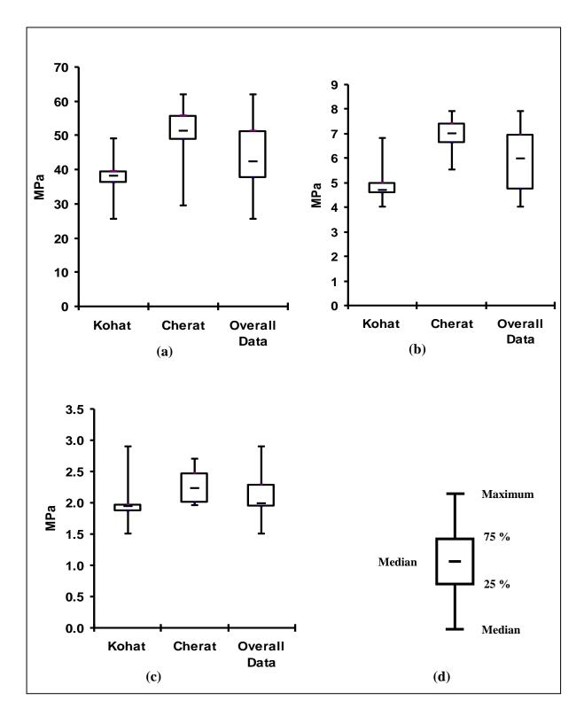
Fig. 1. Statistical analysis of data (a) Uniaxial Compressive Strength (b) Tensile Strength (c) Point Load Index (d) Legend.
