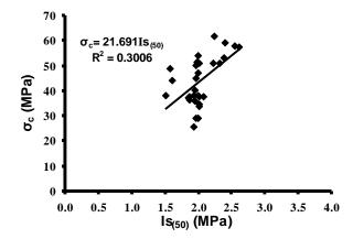
Fig. 3. Relationship between uniaxial compressive and Point load index for limestone from Kohat and Cherat
