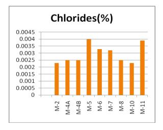
Fig. 6. Chloride content of LWA
