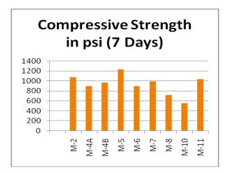
Fig. 7. Compressive strength of LWA
