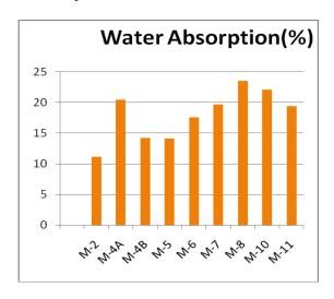
Fig. 2. Water absorption test of LWA
