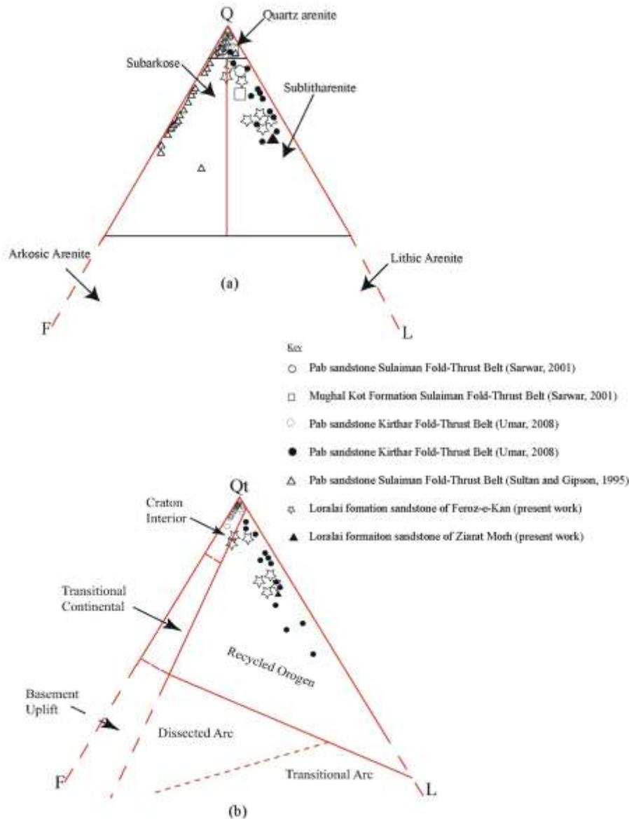
Fig. 6(a). Comparison of Q-F-L plots of sandstone samples of the Upper Cretaceous Pab and Mughal Kot formations of the Sulaiman Fold-Thrust Belt (Sultan and Gipson, 1995; Sarwar, 2001) and Kirthar Fold-Thrust Belt (Umar, 2008) with the Loralai Formation (present work).
