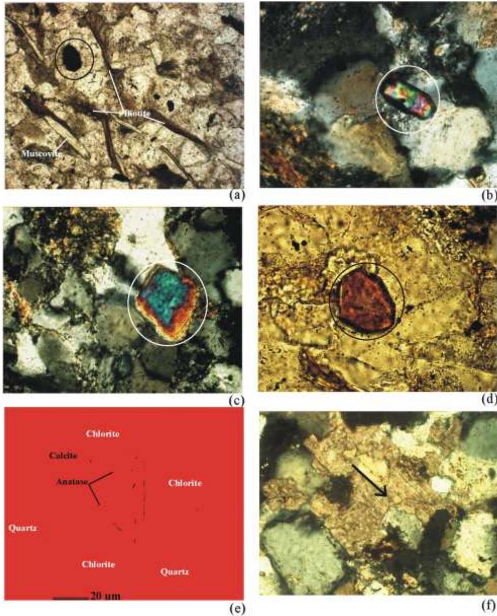
Plate 3. Photomicrographs of sandstone of the Lor Formation showing: (a) muscovite and biotite grains and opaque minerals (circled), 10x10, PPL; (b) zircon grain (circled), 10x40, XPL; (c) tourmaline grain (circled), 10x40, XPL; (d) staurolite grain (circled), 10x40, PPL; (e) back-scattered image showing anatase crystals surrounded by chlorite, 20 µm; (f) extensive replacement of quartz by sparry calcite cement leaving behind the relics of quartz (arrow), 10x25, XPL.
