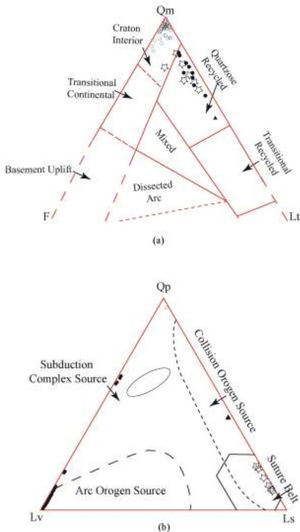
Fig. 7(a). Comparison of the Qm-F-Lt compositional diagram (after Dickinson et al., 1983) of sandstones of the Pab Formation of Kirthar Fold-Thrust Belt (Umar, 2008) with the Loralai Formation (present work).
