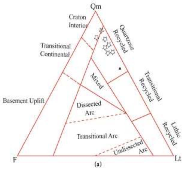
Fig. 4(a). Qm-F-Lt compositional diagram (after Dickinson et al., 1983; Dickinson, 1985) of the sandstone samples of the Lorlai formation.
