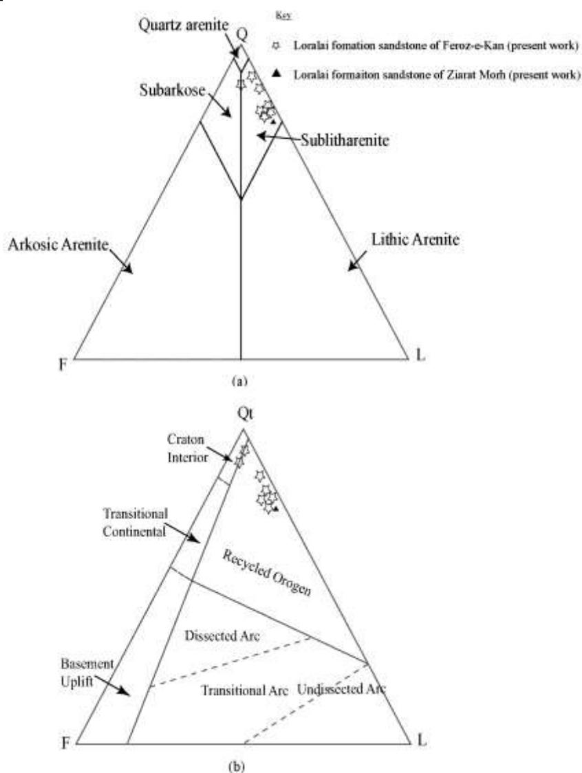
Fig. 3(a). Q-F-L plot of sandstone samples of the Loralai Formation (after Pettijohn et al., 1987).
