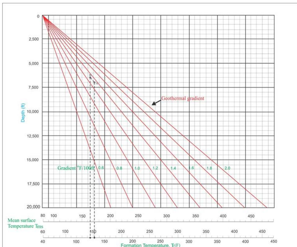
Fig. 14. Determinations of formation temperature through various depths (Schlumberger, 1977).
