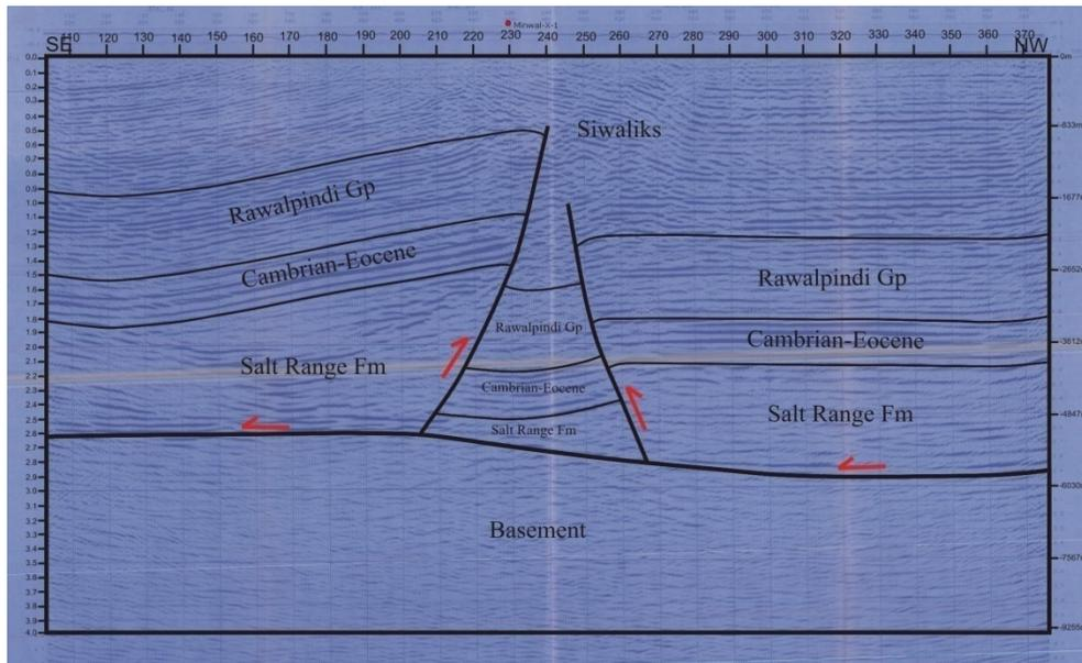
Fig. 9. Seismic section 93-MN-8 showing different reflectors.
