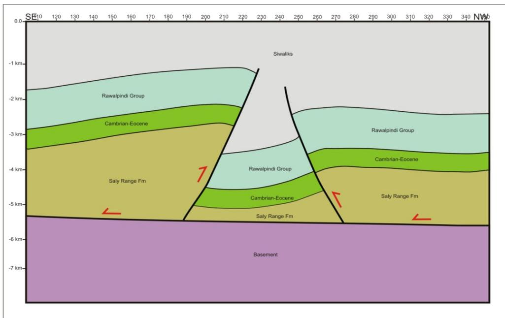
Fig. 8. Depth interpretation of the seismic section 93-MN-6.
