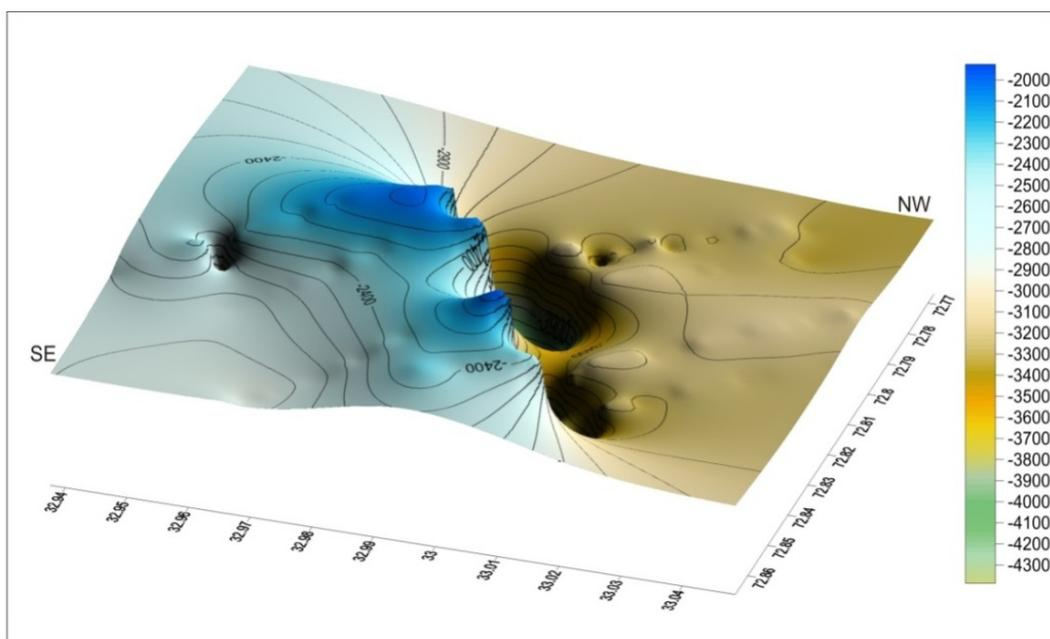
Fig. 13. Depth surface and contour map of the Top Eocene.
