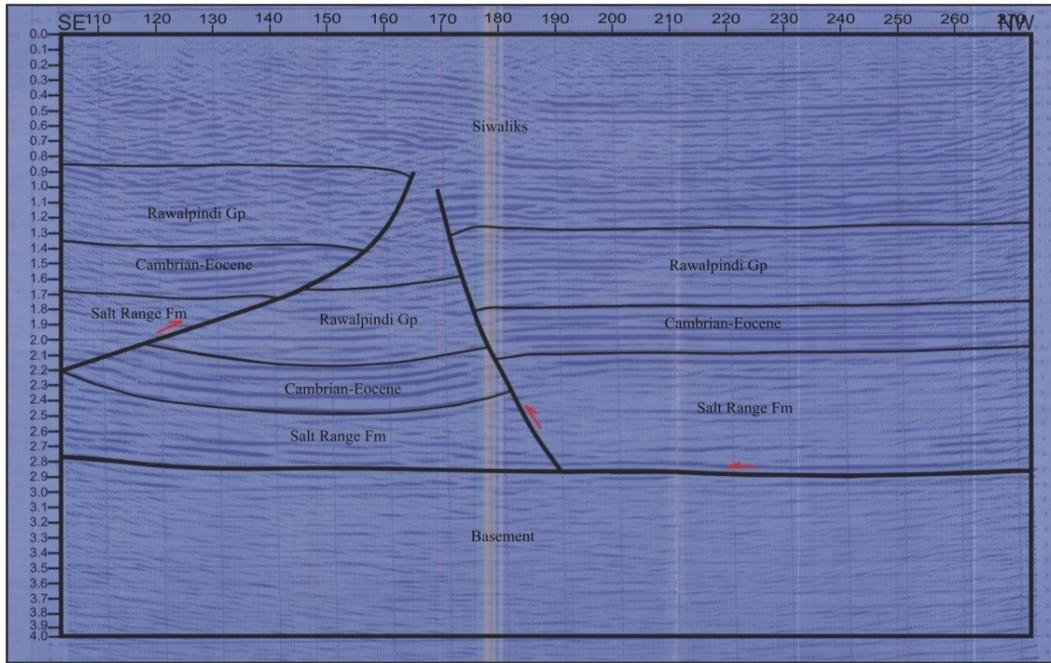
Fig. 11. Seismic section 93-MN-9 showing different reflectors.
