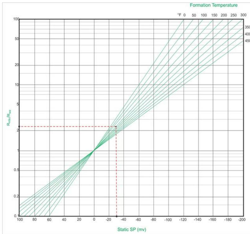
Fig. 16. Determination of  $R_{mf} / R_{we}$  from spontaneous potential (Schlumberger, 1977).
