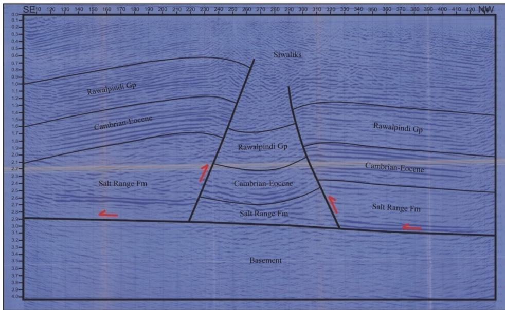
Fig. 4. Seismic section 93-MN-5 showing different reflectors.
