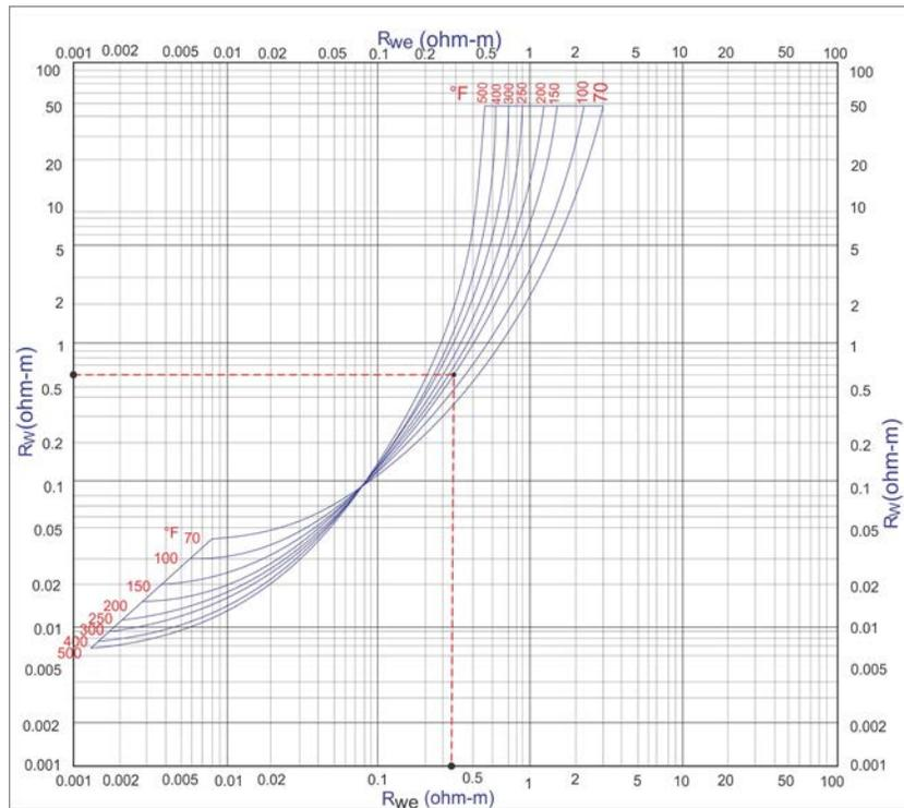
Fig. 17. Determination of  $R_w$  from  $R_{we}$  (Schlumberger, 1977).
