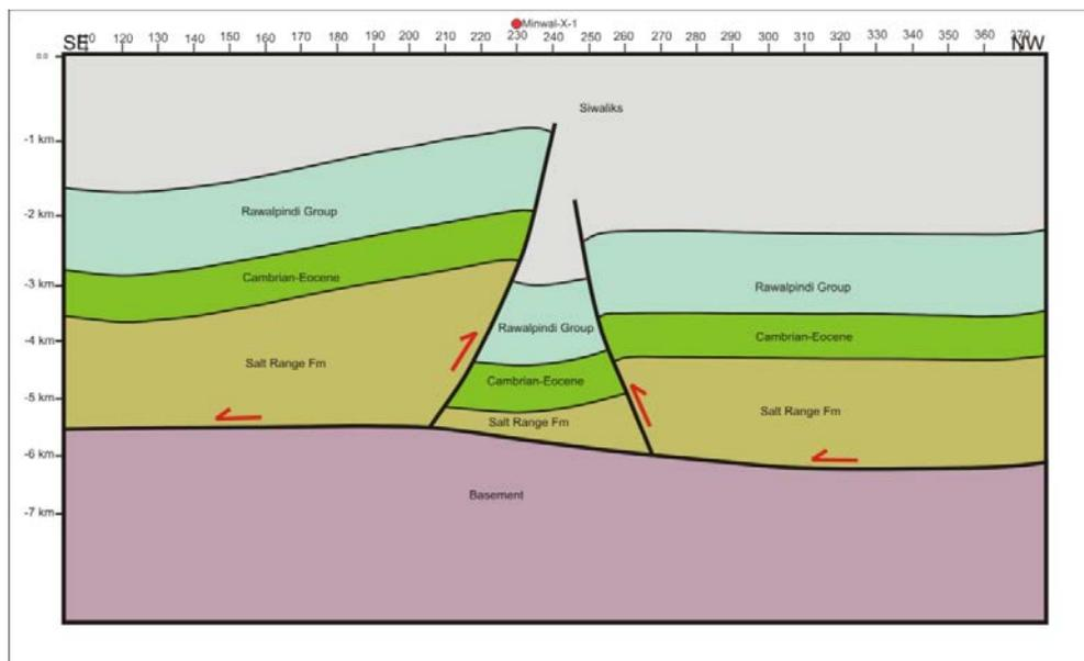
Fig. 10. Depth interpretation of the seismic section 93-MN-8.
