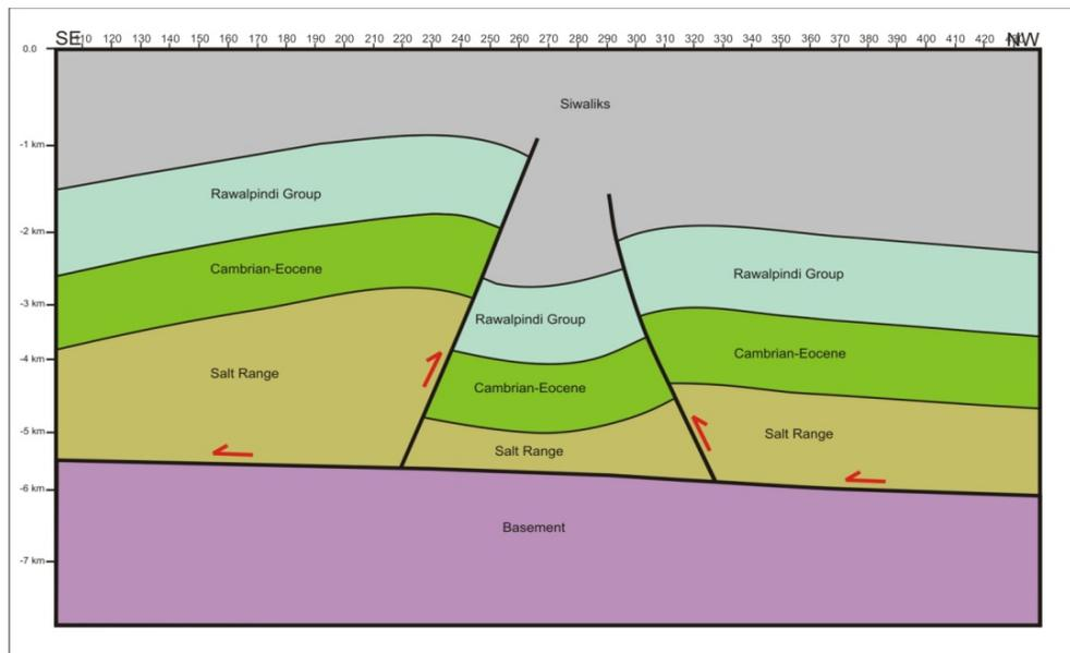
Fig. 6. Depth interpretation of the seismic section 93-MN-5.
