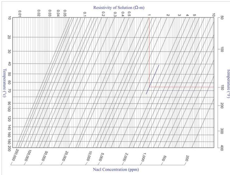
Fig. 15. Correction of  $R_{mf}$  and  $R_{we}$  according to temperature (Schlumberger, 1977).
