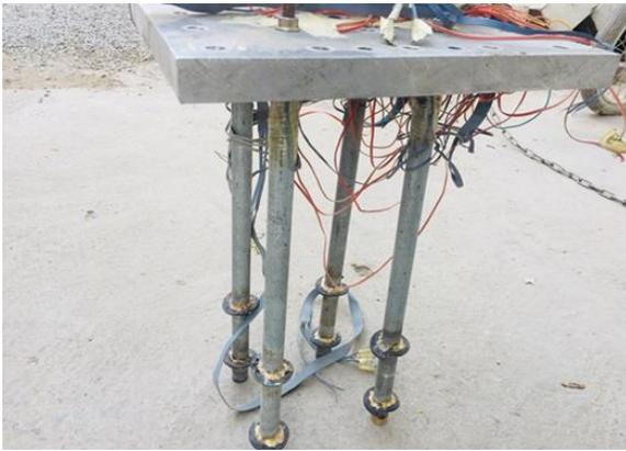
Fig. 8. Pile Raft Setup.
