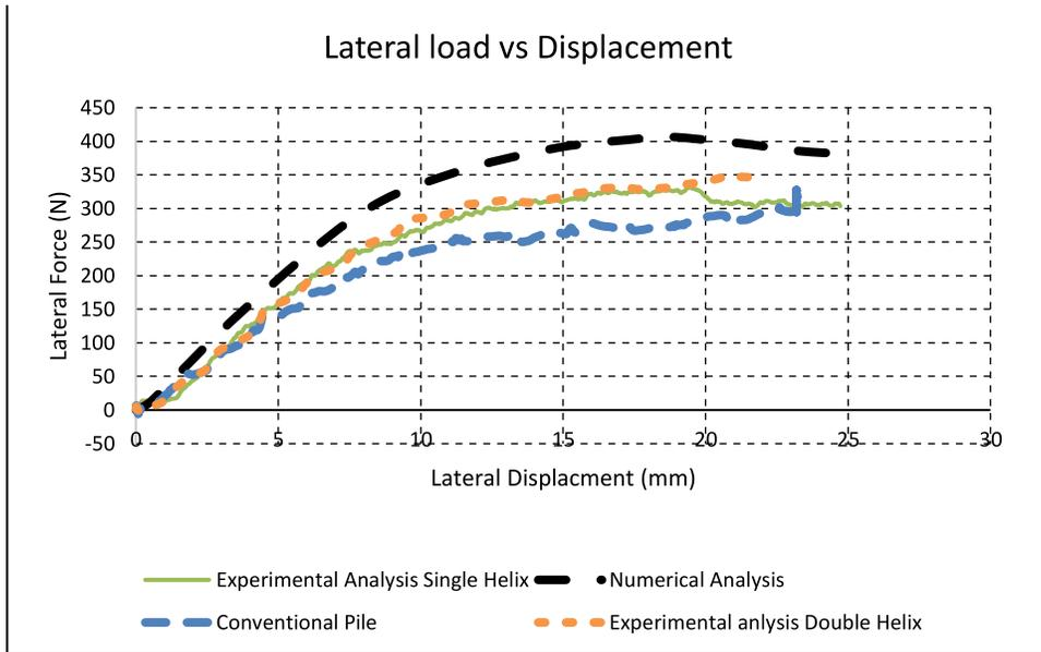
Fig. 21. Comparison of Single Helix and double Single Piles
