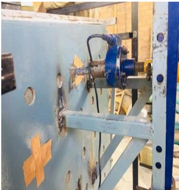
Fig. 12. Lateral Load Cell.
