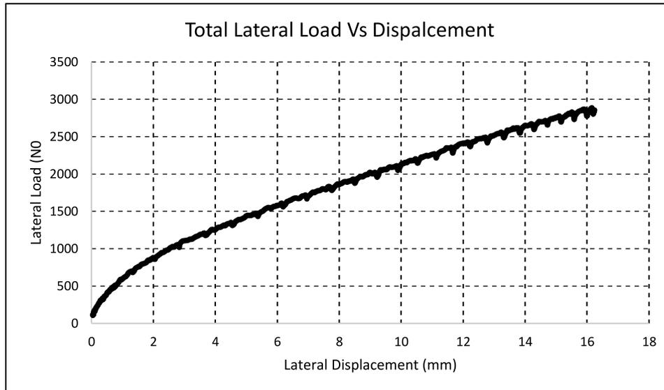
Fig. 23. Total Capacity of Double Helix Four Pile Raft
