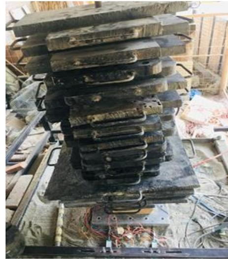
Fig. 15. Axial Building Load 5150N.
