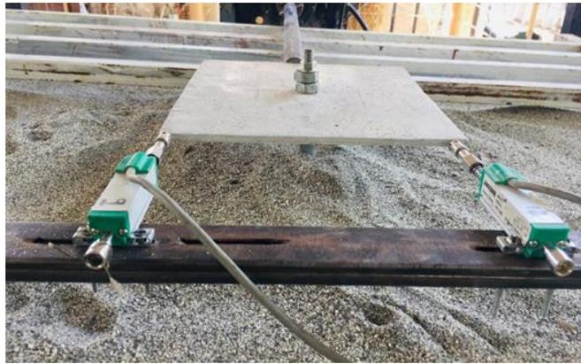
Fig. 9. LVDTs attached to Single Pile with help of Plate.
