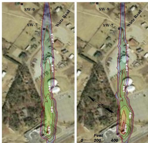
Fig. 17. a) The simulated MTBE plume in deeper zone of the aquifer entered the property area of MS-9 in 1064 days. b) In upper zone, the plume enters after 1096 days.
