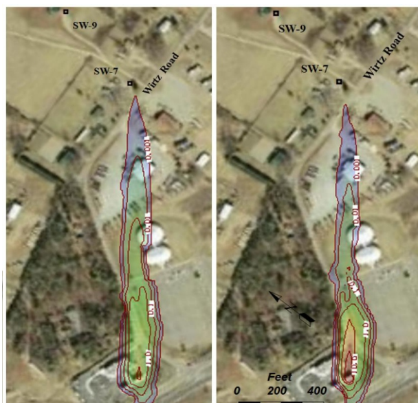
Fig. 16. a) The simulated MTBE plume in deeper zone of the aquifer entered the property area of MS-7 in 810 days. b) In upper zone, the plume enters after 865 days.
