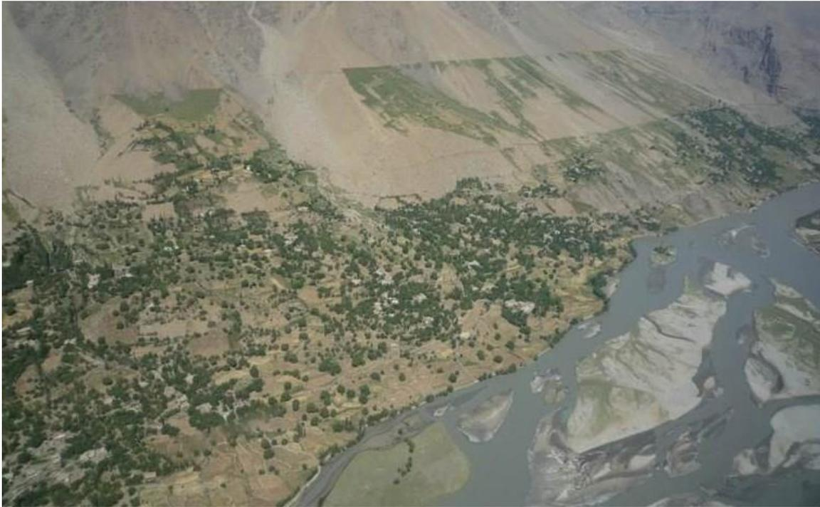
Fig. 11. Non-isolated irrigation channels above settlements and their seepage patterns visible via vegetation. The picture shows the village of Sarchashma 5 km north of Khorog on the Afghan side of the Panj Valley (Fig. 1a).
