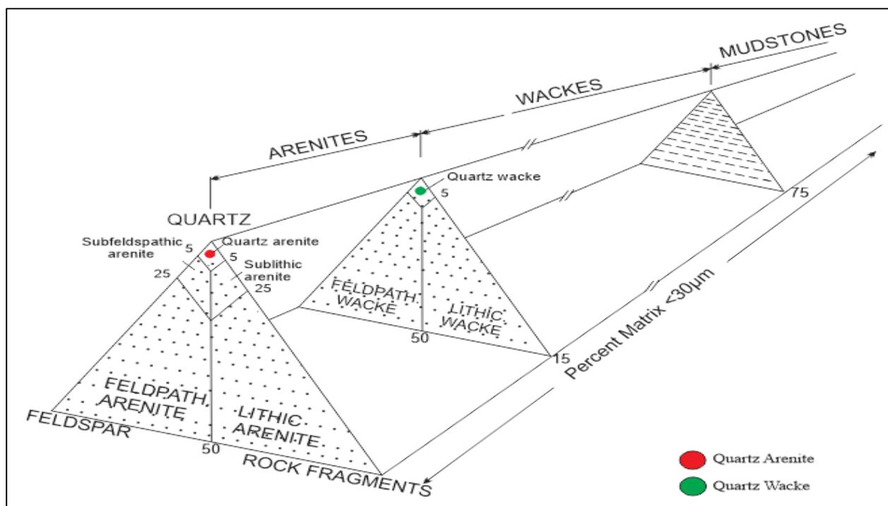
Fig. 5. Shows the model composition of the sandstone units in Lower Cretaceous sequence exposed in TSS and KSS.
