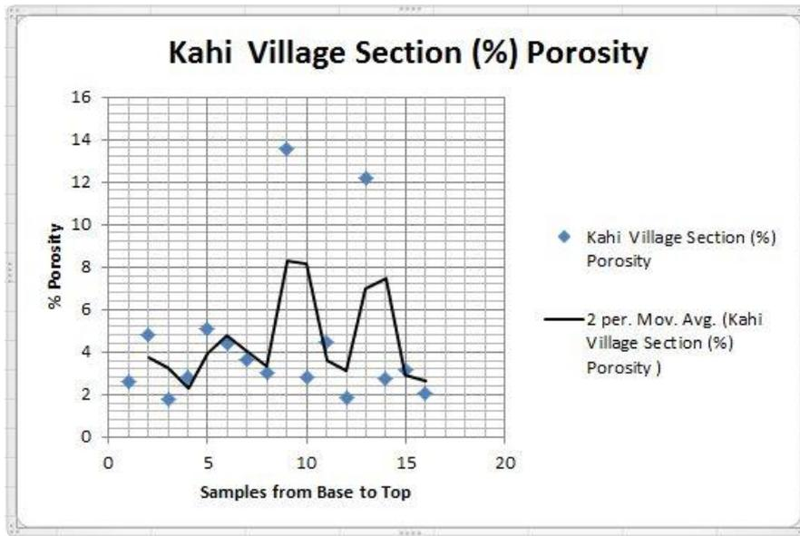
Fig. 12. Shows the porosity curve of Lower Cretaceous sequence in KVS.
