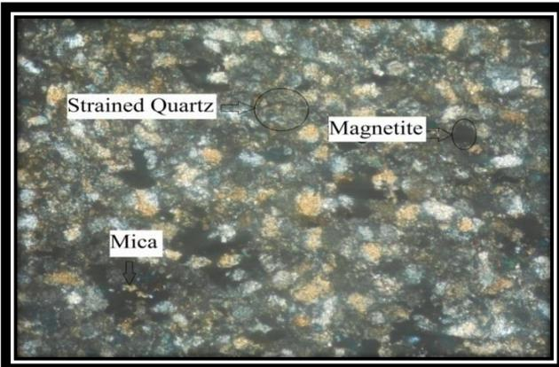
Strained quartz, magnetite and mica in quartzite.
