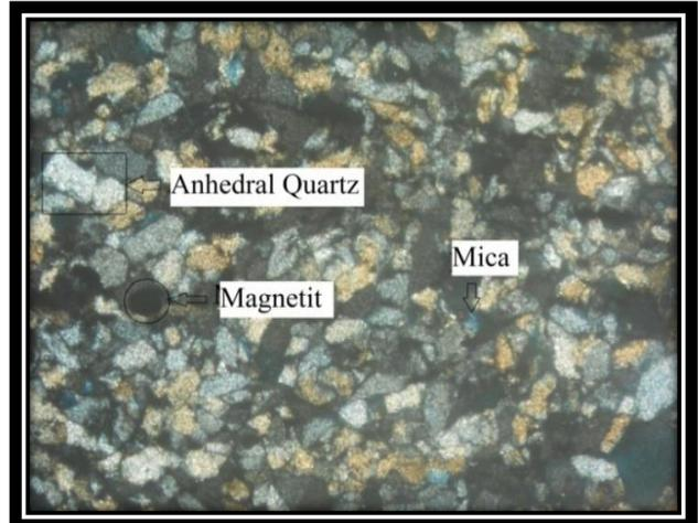
Anhedral quartz, magnetite and mica in quartzite.
