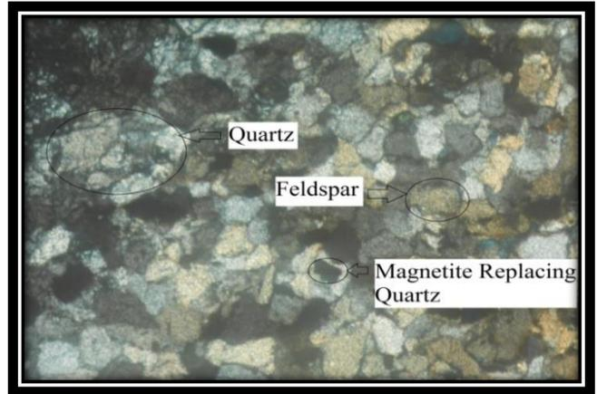
Quartz, feldspar and magnetite replacing quartz in sandstone.
