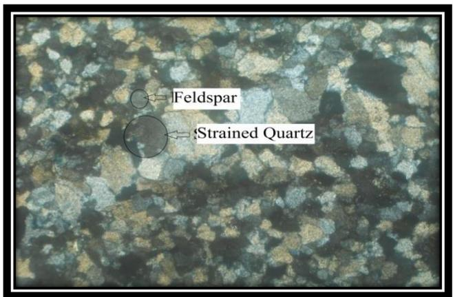
Strained quartz and feldspar in quartz arenite.
