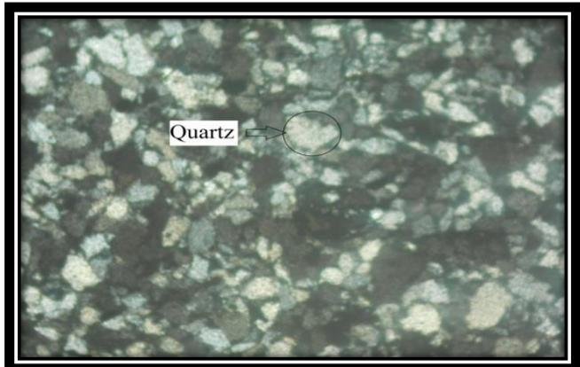
Microphotograph shows quartz in quartzite.
