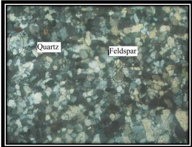
Highly strained quartz and feldspar in quartzite.
