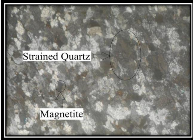
Highly strained quartz and magnetite in schist.
