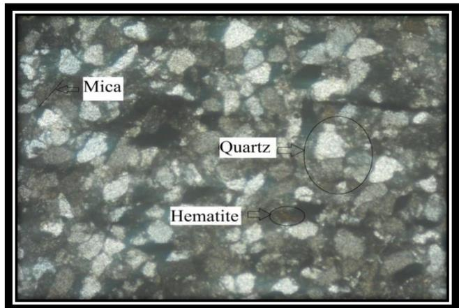
Mica, quartz and hematite in sandstone.
