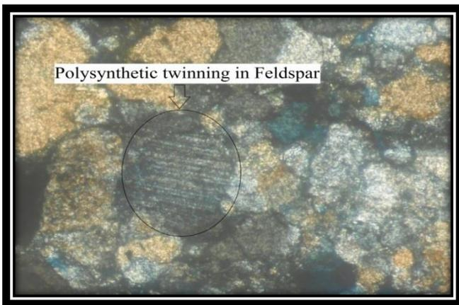
Polysynthetic twinning in plagioclase feldspar in sandstone.
