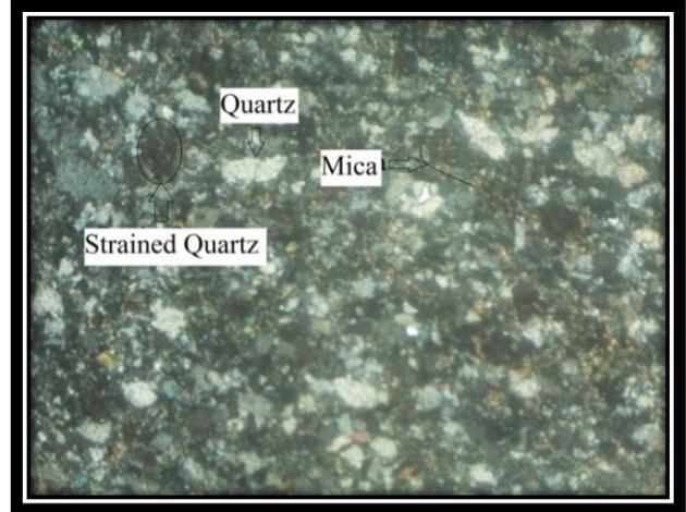
Strained quartz, mica and quartz in schist.
