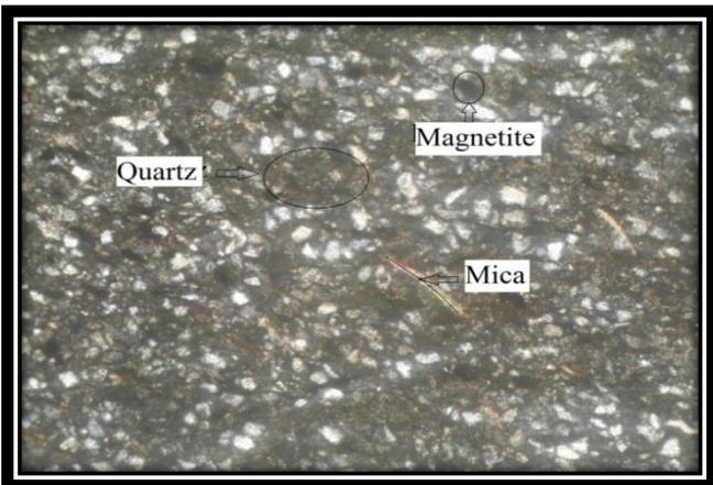
Quartz, magnetite and mica in sandstone
