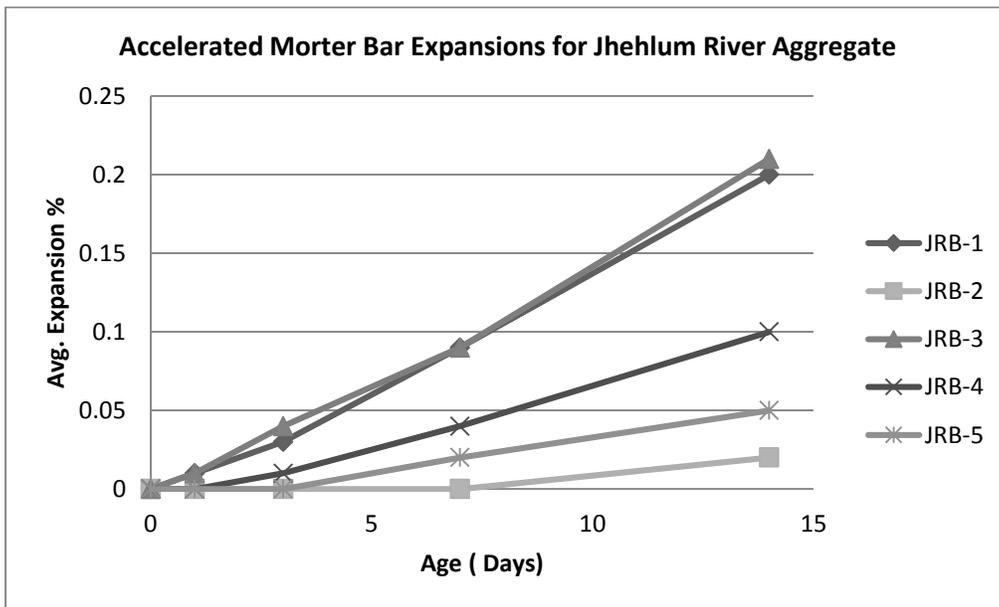
Fig. 3. Accelerated mortar bar expansions for Jhelum river aggregate.
