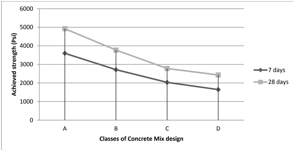
Fig. 2. Achieved strength of normal weight concrete after 7 and 28 days.
