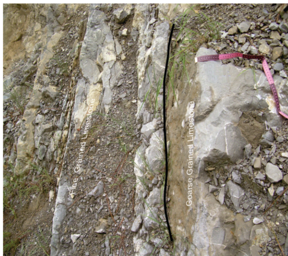
Fig. 5. Contact between medium grained and fine grained limestone.
