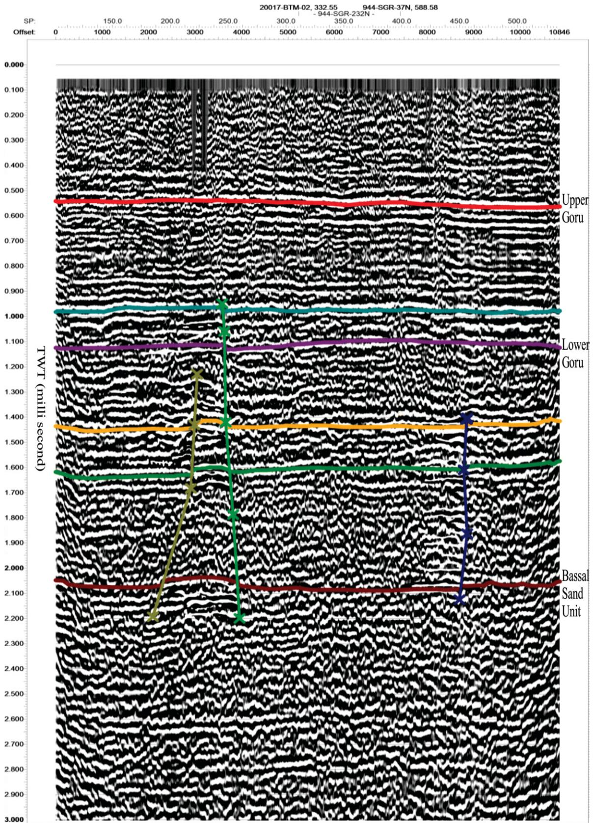
Fig. 5. Seismic time section of seismic line 944-SGR-232 showing time of marked horizons and fault.
