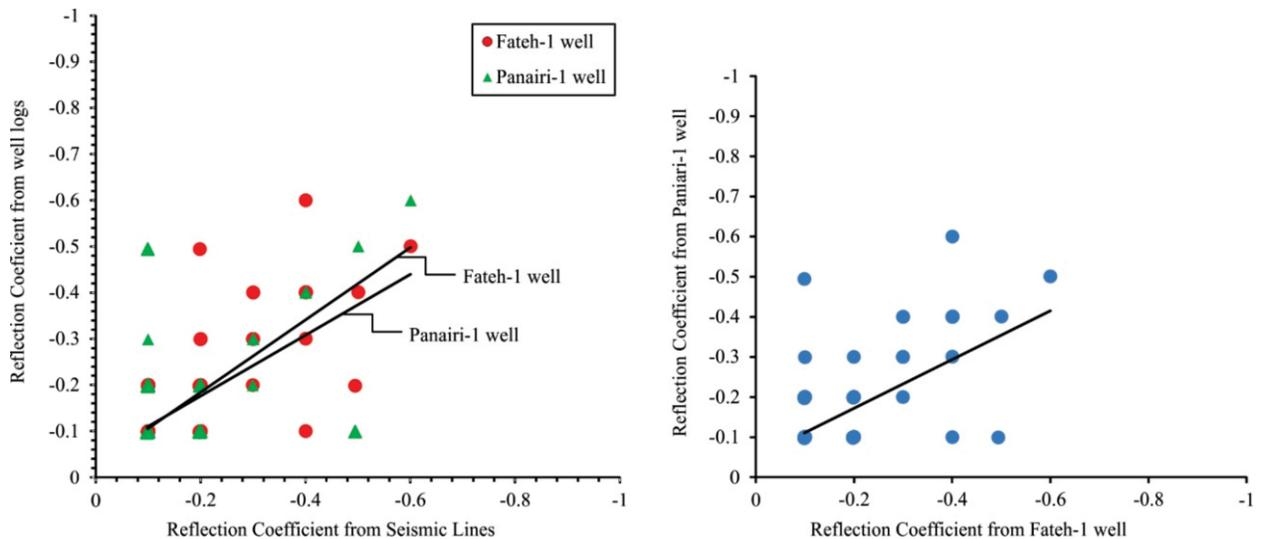
Fig. 6. Correlation of Reflection coefficient from seismic line and well data of Fateh-01 and Panairi-01. A strong correlation of 0.62 results in case of Fateh-01 well, while moderate correlation of 0.43 results in case of Panairi-01 well.
