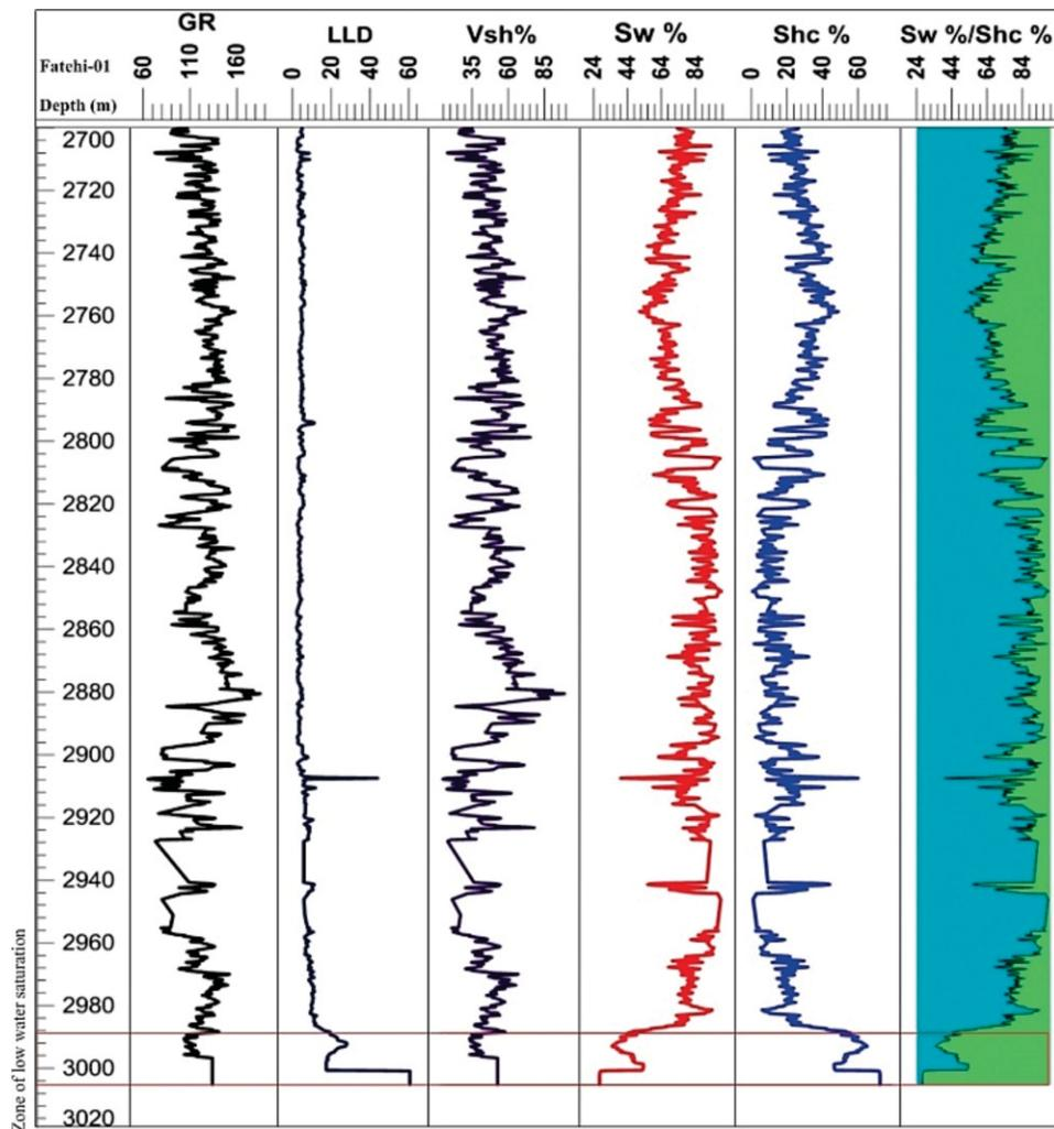
Fig. 7. Petrophysical analysis of Fateh-01 Well, shows variation of different curves with depth and lithology. The zone of low water saturation exist between 2985 to 3005 m.
