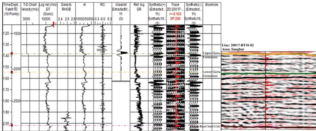
Fig. 2. Horizons and Synthetic seismogram of Fateh-01 Well at 20017- BTM-002. Three horizons Upper Goru, Lower Goru and Basal sand unit are marked using synthetic seismogram (Top, middle and bottom respectively).
