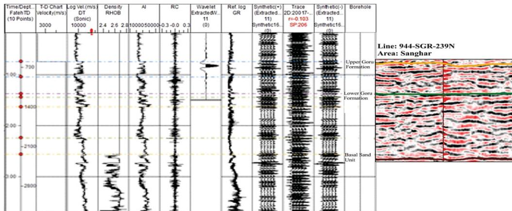
Fig. 3. Horizons and Synthetic Seismogram of Panairi-01 on line 944-SGR-239N. Three horizons Upper Goru, Lower Goru and Basal sand unit are marked using synthetic seismogram (Top, middle and bottom respectively).
