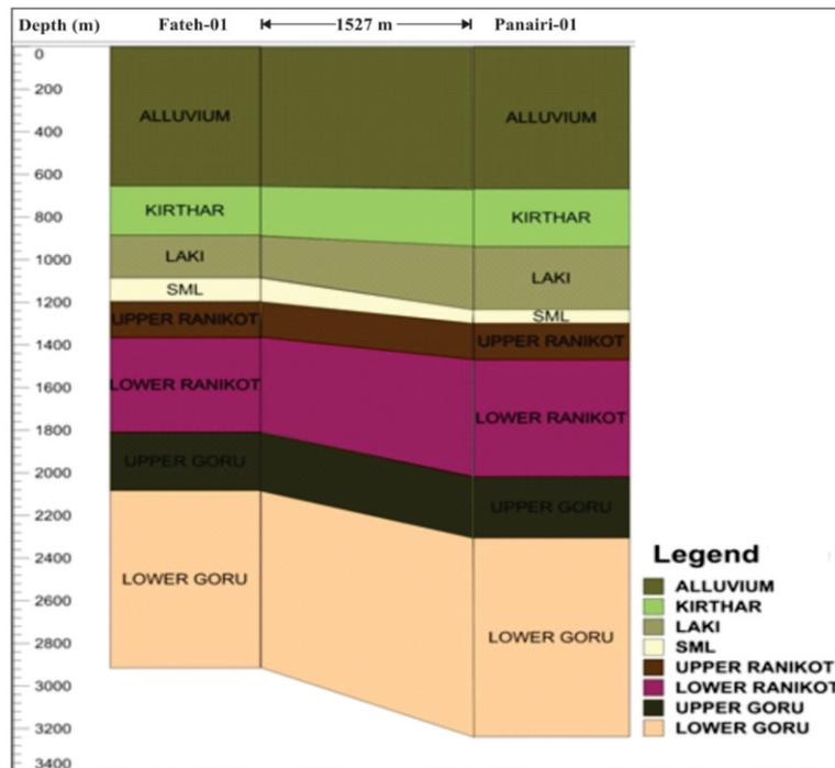
Fig. 9. Geological cross section through Fateh-01 and Panairi-01. Lower Goru Formation has more thickness than other formations in both wells.
