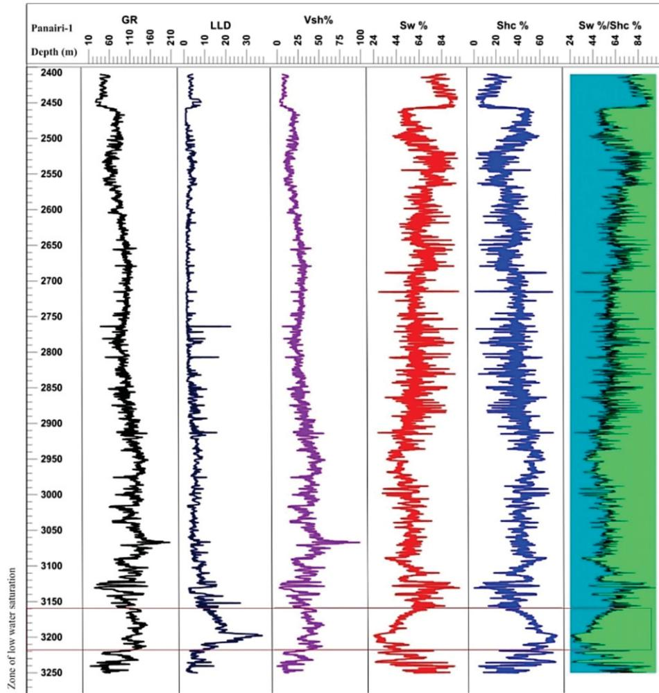
Fig. 8. Petrophysical analysis of Panairi-01 Well, shows variation of different curves with depth and lithology. The zone of low water saturation exist between 3152 to 3210 m.
