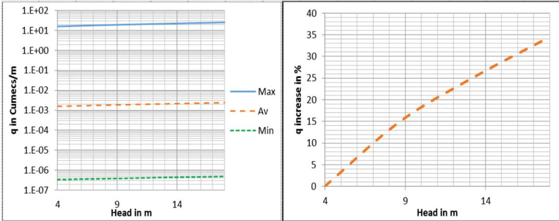
Fig. 8. Reservoir Head VS seepage quantity (a) for three analysis types (b) Plot of Average analysis.
