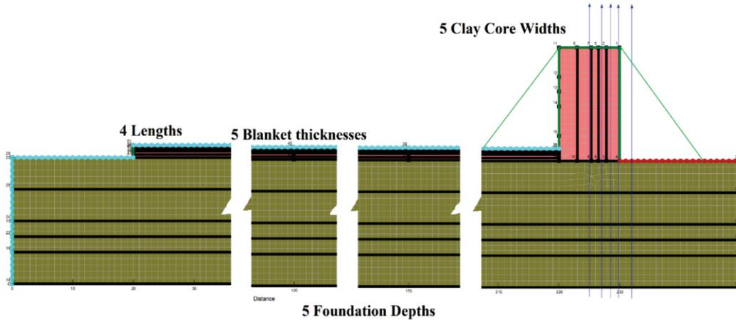
Fig. 3. Basic analysis model for Sensitivity study of parameters.
