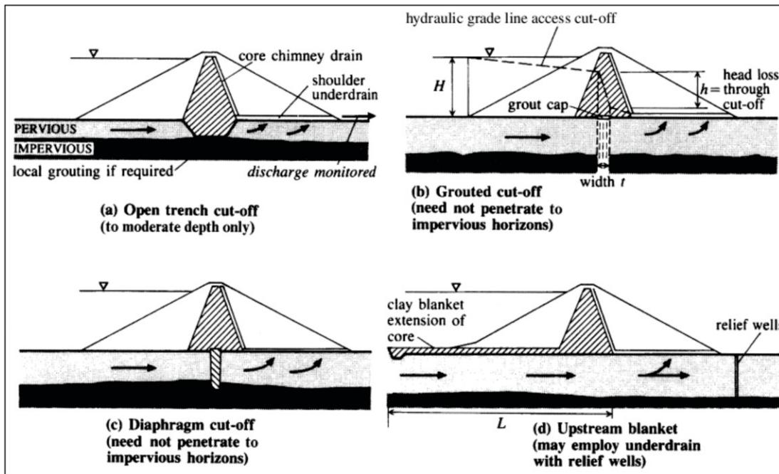
Fig. 1. Foundation Seepage Control methods (ICOLD).
