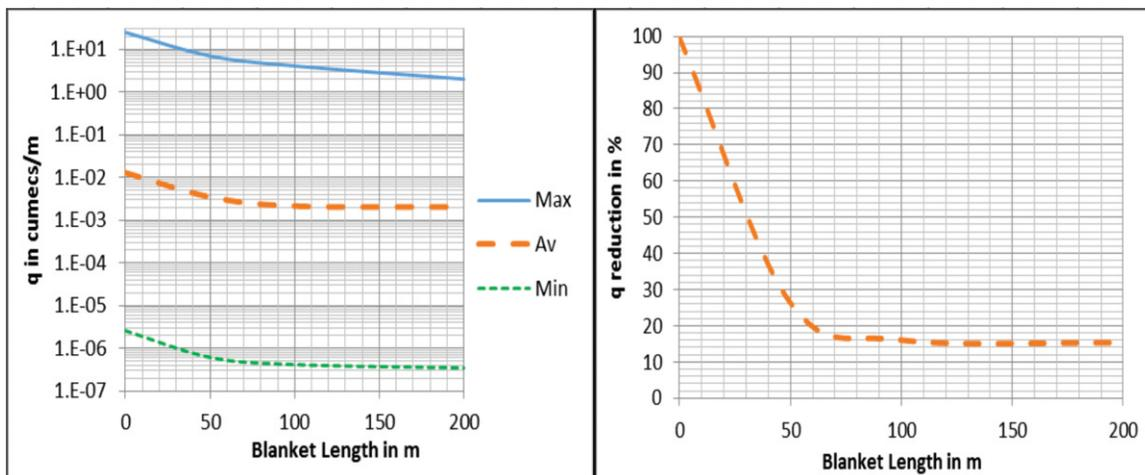
Fig. 4. Blanket Length Vs seepage (a) for three analysis types (b) Plot of Average analysis.
