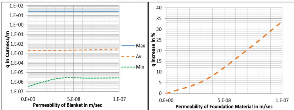
Fig. 10. Permeability of Blanket material Vs seepage quantity (a) for three analysis types (b) Plot of Average analysis.
