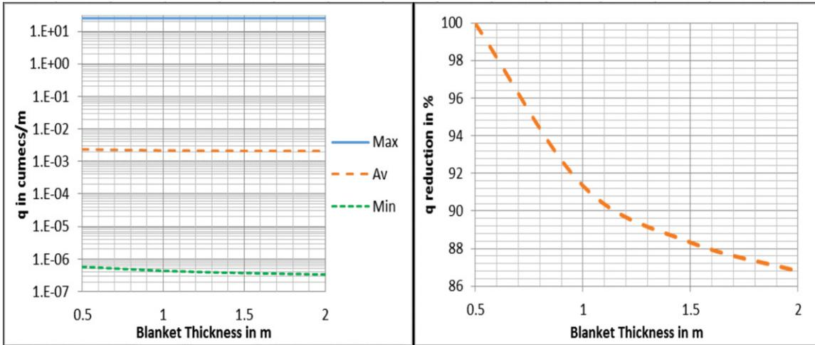
Fig. 5. Blanket Thickness Vs seepage quantity (a) for three analysis types (b) Plot of Average analysis.
