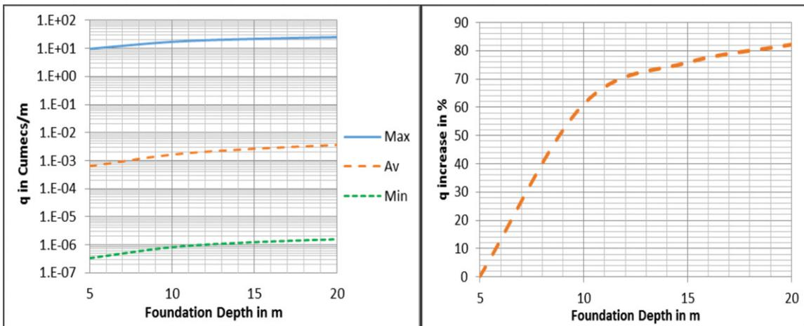
Fig. 7. Foundation bed depth Vs seepage quantity (a) for three analysis types (b) Plot of Average analysis.
