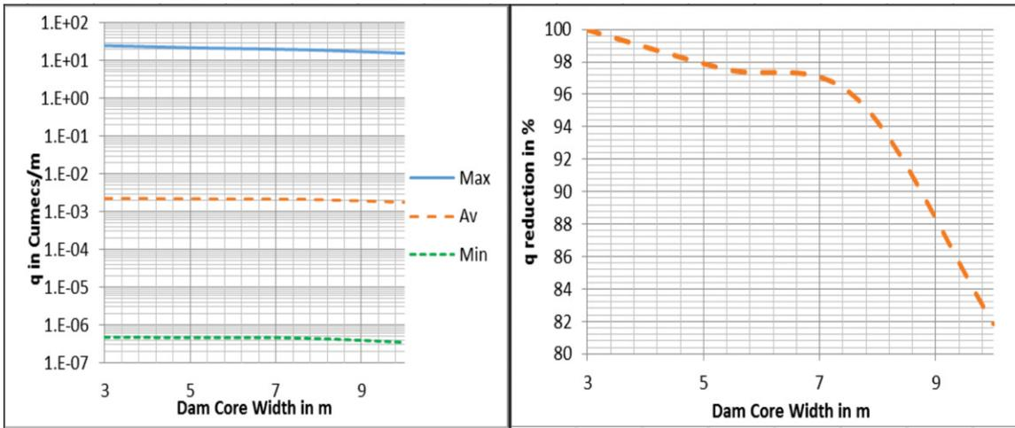
Fig. 6. Dam core Width Vs seepage quantity (a) for three analysis types (b) Plot of Average analysis.
