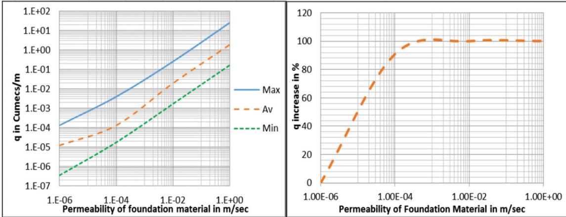
Fig. 9. Permeability of foundation material Vs seepage quantity (a) for three analysis types (b) Plot of Average analysis.
