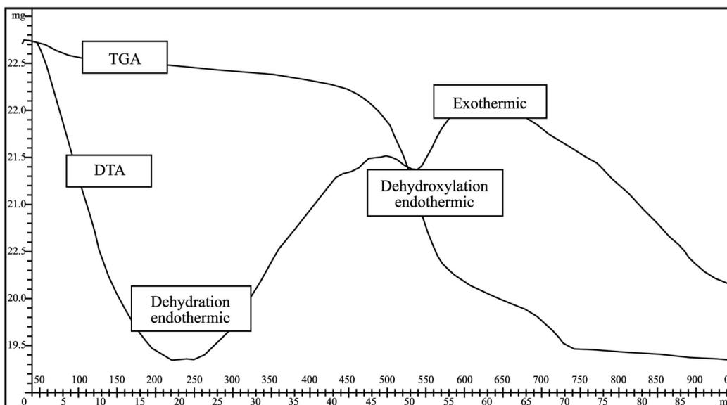
Fig. 4. DT and TGA graph of kaolin (raw) sample of Nagar Parkar deposit.
