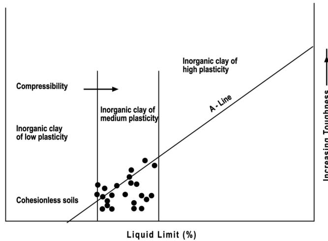
Fig. 3a. Plasticity chart for the classification of Nagar Parkar Kaolin deposit (after Casagrande, 1948).
