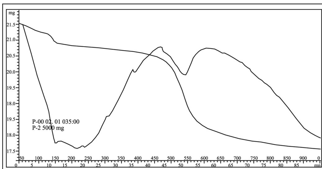
Fig. 5. DT-TGA curve of kaolin (washed) sample of Nagar Parkar
