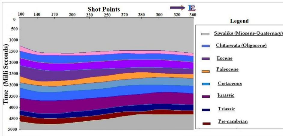
Fig. 7. Time section of 914-RPR-05 (Kotrum Structure)
