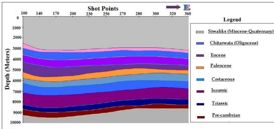
Fig. 8. Geoseismic model of 914-RPR-05 (Kotrum Structure)
