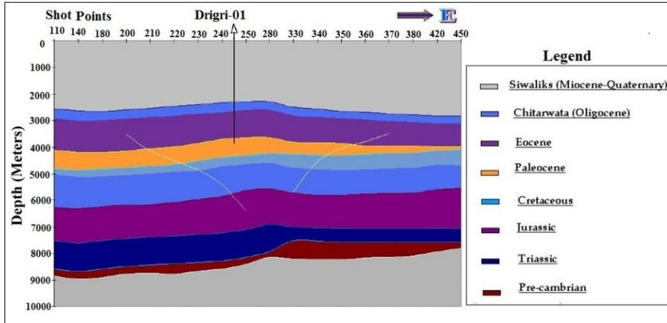
Fig. 6. Geoseismic model of 914-RPR-03 (Drigri Anticline)
