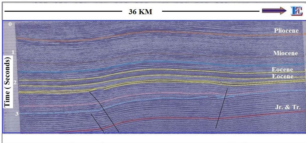
Fig. 10. Interpreted Seismic section of 914-RPR-03 showing Drigri Anticline (36 km)
