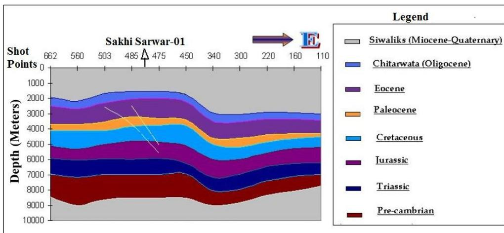
Fig. 4. Geoseismic model of 976-FZP-06 (Sakhi Sarwar Anticline).
