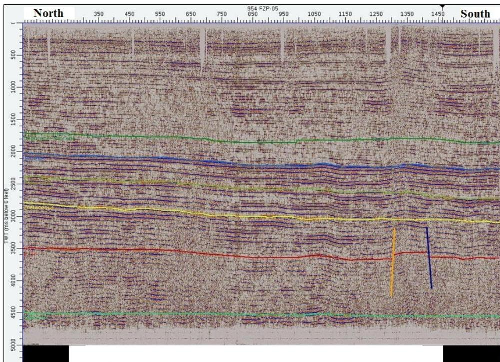
Fig. 11. Interpreted Seismic section of 954-FZP-05 (north-south orientation)
