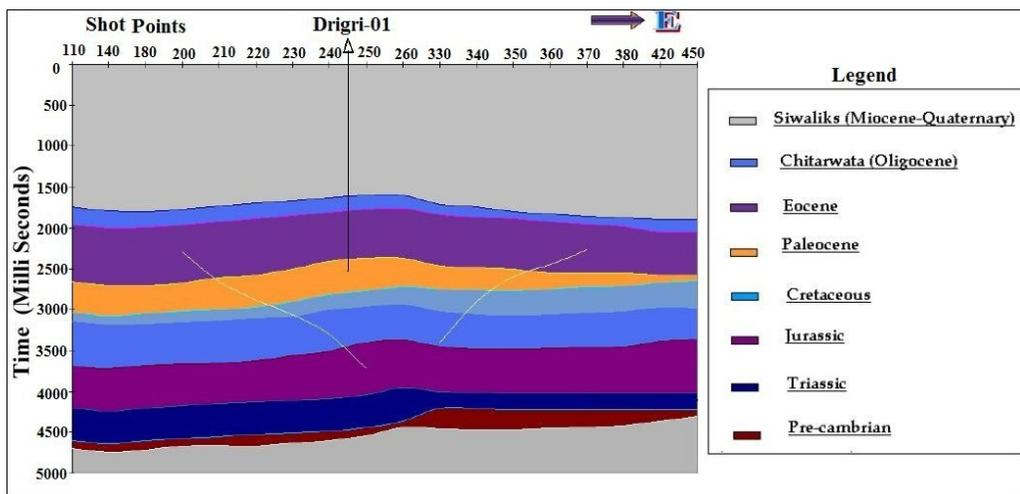
Fig. 5. Time section of 914-RPR-03 (Drigri Anticline)
