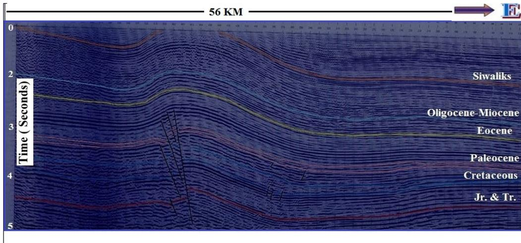
Fig. 9. Interpreted Seismic section of 976-FZP-06 showing Sakhi Sarwar Anticline (56 km).
