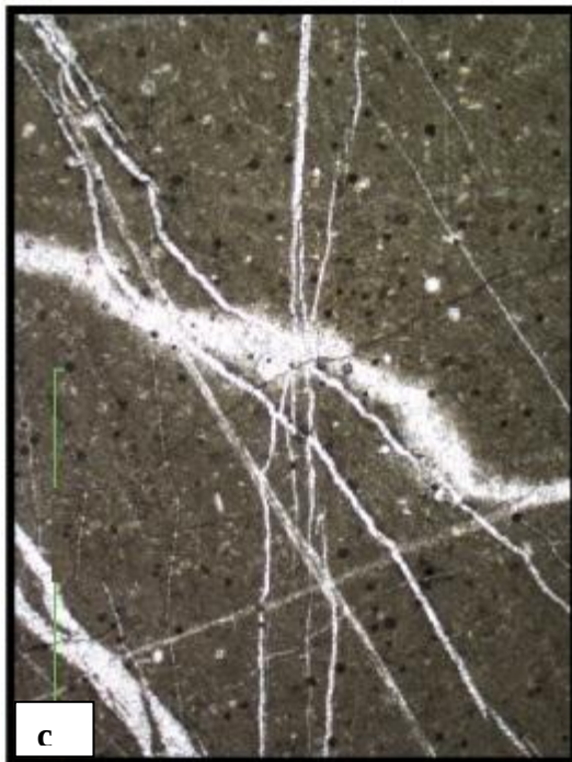
Fig. 6. The composite photomicrographs showing microcracks and calcite veins present in the Kohat Limestone of the research area. Figs. (a) and (b) are showing intense microcracks, and (c) and (d) are showing dominant veins in PPL and XPL, respectively. Scale for all the above microphotographs is 1mm.
